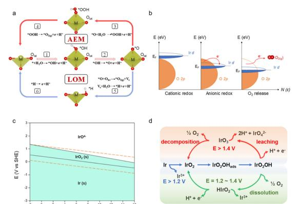
Fig. 1 (a) Schematic representation of the adsorbate evolving mechanism (AEM) and lattice oxygen mechanism (LOM); the four electrochemical reaction steps for each mechanism are shown with "\*" and Vo denotes the lattice oxygen vacancy, respectively. M stands for the metal (Ir); (b) schematic representation of the energy level versus density of states N(s); (c) pH-potential diagram of Ir. (d) Universal mechanism for Ir catalysts correlating both the OER and dissolution pathways.
