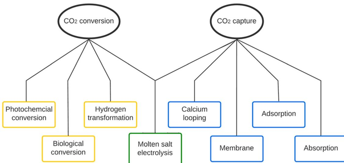
Fig. 3 General CO<sub>2</sub> capture methods developed.
