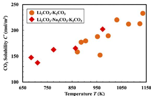
Fig. 7 CO<sub>2</sub> solubility in molten carbonates at different temperatures at 1.01 × 10<sup>5</sup> Pa.<sup>87</sup>
