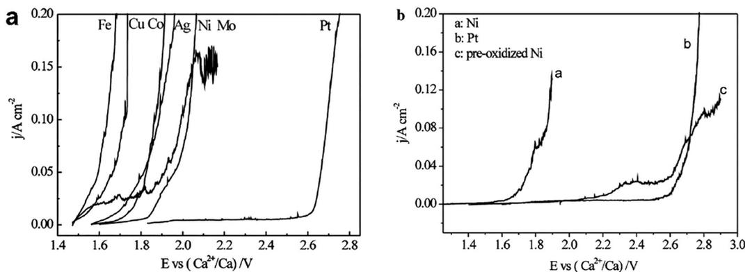
**Fig. 11** (a) Polarization curves of metals in molten  $\text{CaCl}_2 - 2.5\text{ mol}\% \text{ CaO}$  at  $850\text{ }^\circ\text{C}$  (potential scan rate,  $2\text{ mV s}^{-1}$ ); (b) polarization curves of Ni, Pt and pre-oxidized Ni in molten  $\text{CaCl}_2$  at  $850\text{ }^\circ\text{C}$  (potential scan rate,  $2\text{ mV s}^{-1}$ ).<sup>103</sup>
