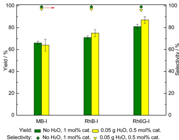
**Fig. 4** Effect of using H<sub>2</sub>O as an HBD on the catalytic activity of dye-I (dye = MB, RhB, Rh6G) combined with a lower catalyst loading relative to the epoxide (0.5 mol% in tests with H<sub>2</sub>O, 1 mol% in tests without H<sub>2</sub>O). Reaction conditions: styrene oxide (20 mmol), *o*-xylene (1.5 mmol) as internal standard, 80 °C, 10 bar CO<sub>2</sub>, 24 h.
