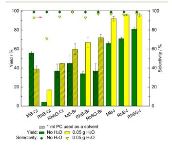
Fig. 3 Effect of using H<sub>2</sub>O as an HBD on the catalytic activity of (ionexchanged) dyes as organocatalysts for the conversion of styrene oxide and CO2 into styrene carbonate. Reaction conditions: styrene oxide (20 mmol), organic catalyst (1 mol% relative to the epoxide), o-xylene (1.5 mmol) as internal standard, 80 °C, 10 bar CO<sub>2</sub>, 24 h.
