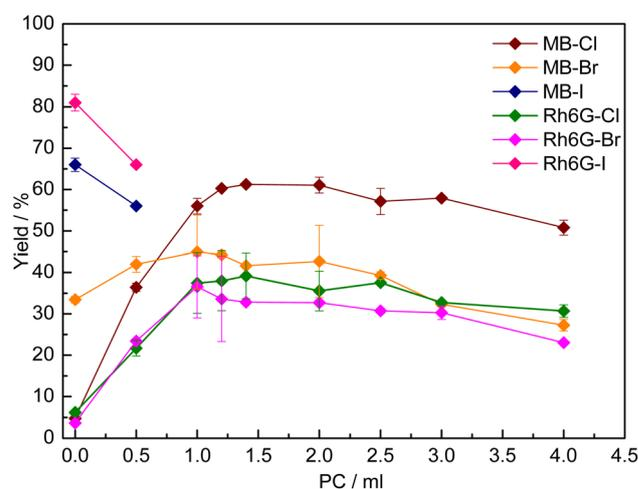
**Fig. 2** Effect of the use of propylene carbonate (PC) as a solvent on the catalytic activity of MB-X and Rh6G-X (X = Cl, Br, I) in the reaction of  $CO_2$  with styrene oxide. Reaction conditions: styrene oxide (20 mmol), organocatalyst (1 mol% relative to the epoxide), *o*-xylene (1.5 mmol) as internal standard, 80 °C, 10 bar  $CO_2$ , 24 h.
