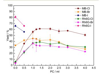
Fig. 2 Effect of the use of propylene carbonate (PC) as a solvent on the catalytic activity of MB-X and Rh6G-X (X = Cl, Br, I) in the reaction of  $CO_2$  with styrene oxide. Reaction conditions: styrene oxide (20 mmol), organocatalyst (1 mol% relative to the epoxide), o-xylene (1.5 mmol) as internal standard, 80 °C, 10 bar  $CO_2$ , 24 h.
