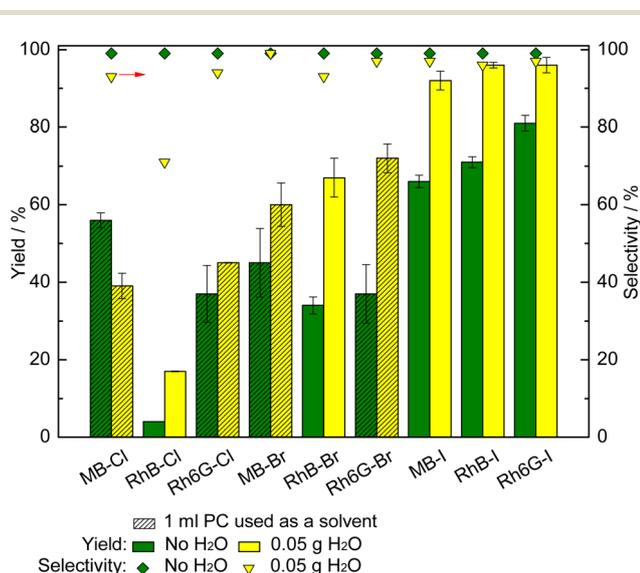
**Fig. 3** Effect of using H<sub>2</sub>O as an HBD on the catalytic activity of (ion-exchanged) dyes as organocatalysts for the conversion of styrene oxide and CO<sub>2</sub> into styrene carbonate. Reaction conditions: styrene oxide (20 mmol), organic catalyst (1 mol% relative to the epoxide), *o*-xylene (1.5 mmol) as internal standard, 80 °C, 10 bar CO<sub>2</sub>, 24 h.
