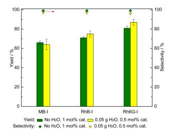
Fig. 4 Effect of using  $H_2O$  as an HBD on the catalytic activity of dye-l (dye = MB, RhB, Rh6G) combined with a lower catalyst loading relative to the epoxide (0.5 mol% in tests with  $H_2O$ , 1 mol% in tests without  $H_2O$ ). Reaction conditions: styrene oxide (20 mmol), o-xylene (1.5 mmol) as internal standard, 80 °C, 10 bar  $CO_2$ , 24 h.
