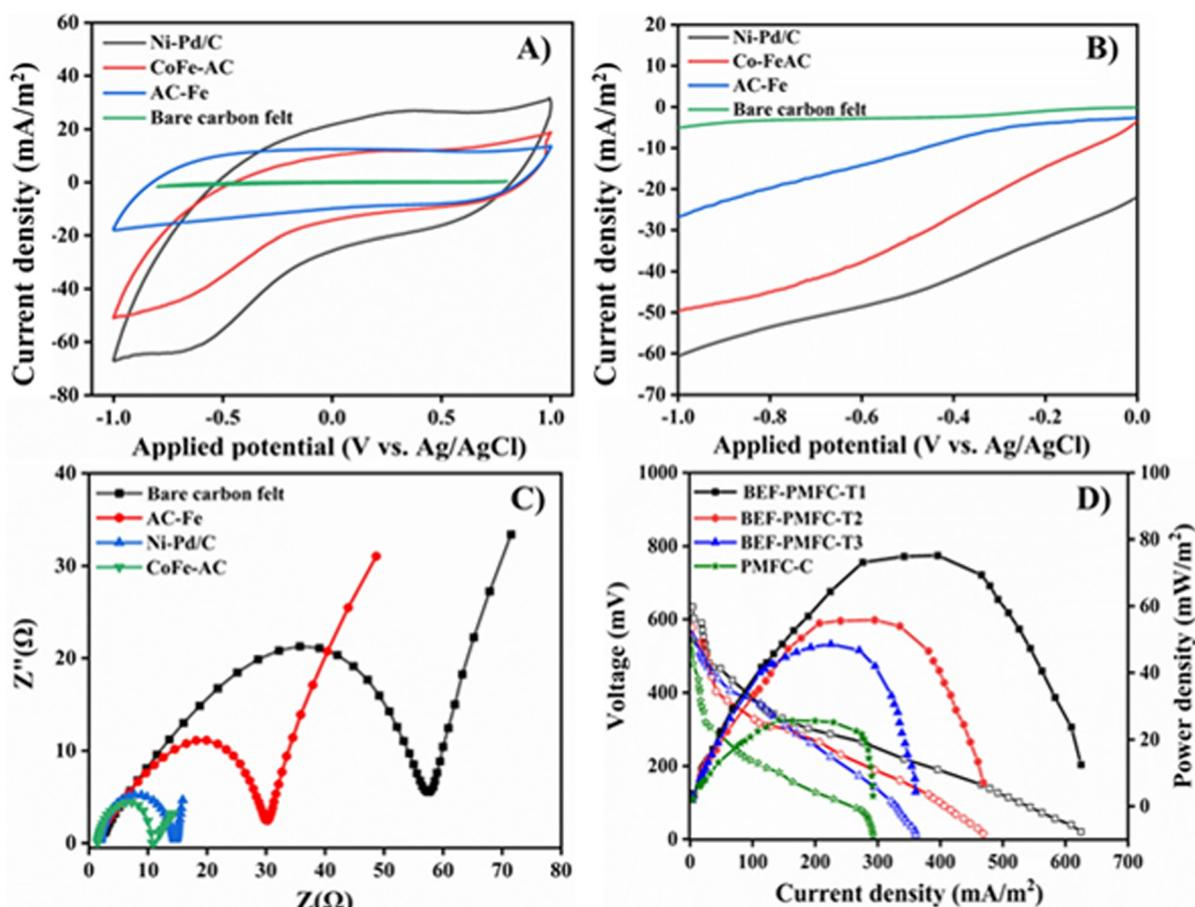
**Fig. 10** (A) The CV and (B) LSV analysis of Ni-Pd/C, CoFe-AC, and AC-Fe catalysts in comparison with bare carbon felt; (C) the Nyquist plots of bare carbon felt and different catalyst-coated electrodes during the EIS test; and (D) polarisation curves of different catalyst-coated BEF-PMFC.
