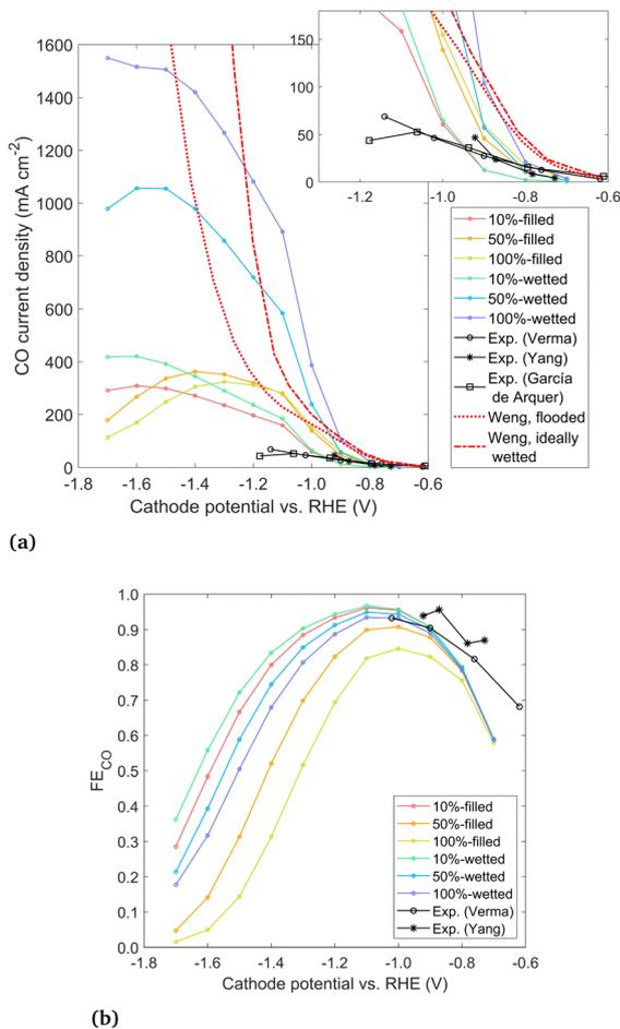
Fig. 7 (a) Geometric CO current density for modeled cases and experimental data from Verma *et al.*,<sup>38</sup> Yang *et al.*,<sup>4</sup> and Garcia de Arquer *et al.*<sup>24</sup> and (b) overall Faradaic efficiency to CO.
