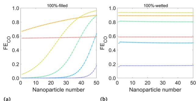
Fig. 6 Mean  $FE_{CO}$  at the surface of each nanoparticle for (a) the 100%-filled case and (b) the 100%-wetted case, at various applied potentials. Nanoparticles are numbered starting at 1 for the left-most (deepest) particle. (Legend same as Fig. 5)
