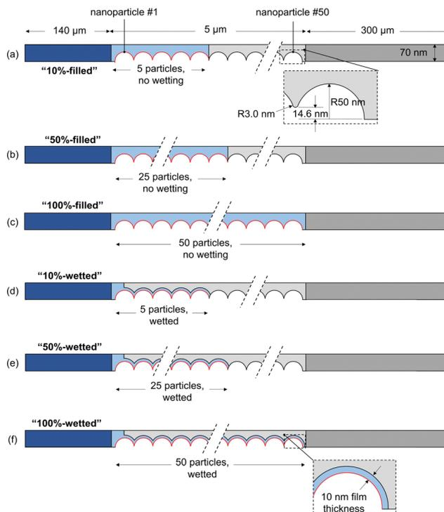
Fig. 3 Geometry and wetting configuration for three filled (a–c) and three wetted (d–f) GDE cases, with abbreviated names in bold and the catalyst surface active for CO<sub>2</sub>R shown in red.
