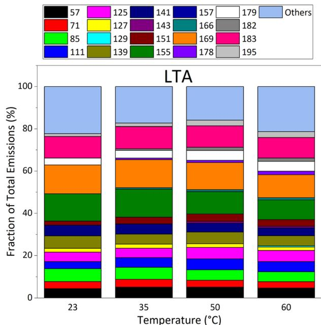
Fig. 5 Evolution of VOC emission composition in % for the 20 masses exhibiting the strongest contributions ( $EF > 22 \mu\text{g m}^{-2} \text{h}^{-1}$  at  $60 \text{ }^\circ\text{C}$ ) as a function of temperature, as measured by PTR-ToFMS under dry ( $RH = 0.1\%$ ) and dark conditions, for the LTA2 old asphalt sample.
