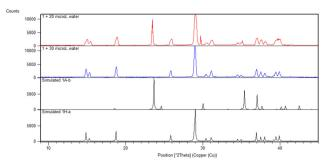
Fig. 1 PXRD pattern of 1 sublimed with 20  $\mu L$  water (red) and 30  $\mu L$ water (blue), compared to simulated patterns (black) for the anhydrous and hydrate crystals.
