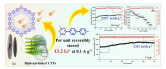
Fig. 7 Schematical illustration of the structure of a biphenyl-based CTF and its electrochemical performance. Reproduced from ref. 127 with permission from Elsevier, Copyright 2022.
