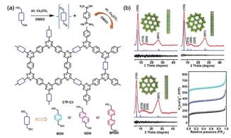
Fig. 3 (a) Pathways for the synthesis of the crystalline CTFs. (b) XRD patterns and N<sub>2</sub> adsorption and desorption isotherms of crystalline CTFs. Reproduced from ref. 65 with permission from Wiley-VCH, Copyright 2018
