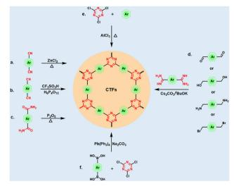
Fig. 2 Synthetic reactions and routes for the preparation of CTFs, including ionothermal method, superacid-catalyzed trimerization,  $P_2O_5$ -catalyzed method, strong base-catalyzed polycondensation, Friedel-Crafts reactions and C-C coupling reactions
