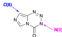
Fig. 4 Accessible sites of modification of the imidazotetrazine scaffold.
