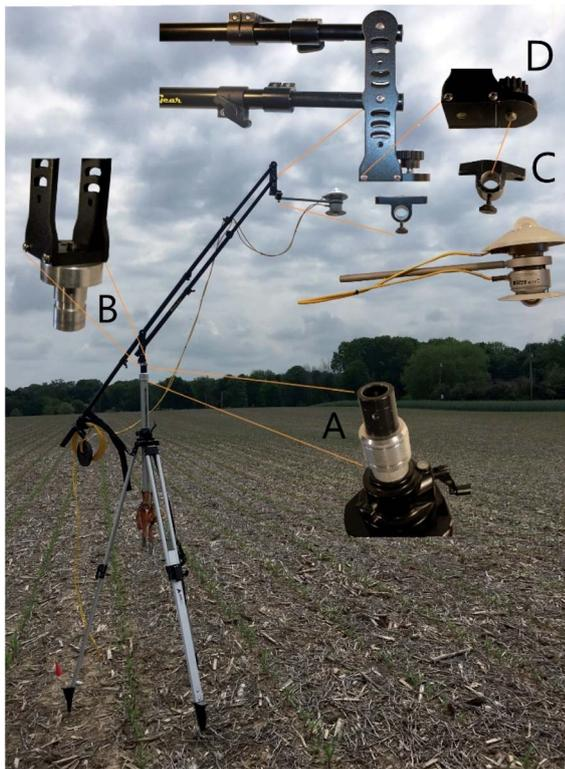
Fig. 1 Portable apparatus for measuring *in situ* albedo at Site 1. The height of the albedometer is raised or lowered through a combination of tripod leg adjustments and changing the angle of the sensor boom. A threaded spud socket (A) on the tripod and swivel spud (B) allows adjustment of the sensor boom. A rod clamp (C) is attached to sensor boom with machined, hand-tightening bolt (D).
