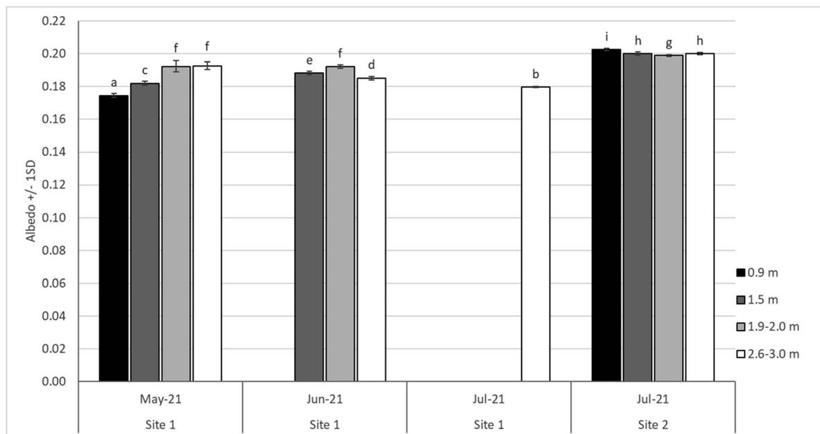
Fig. 5 Mean albedo measured at different sensor heights and growing season dates in corn (Site 1) and hay (Site 2) crops. Letters indicate statistical difference at  $\alpha = 0.05$  using repeated measures factorial ANOVA followed by Tukey HSD. At Site 1, data was excluded for low (June) and low, medium, and high (July) sensor heights because corn height exceeded sensor height.
