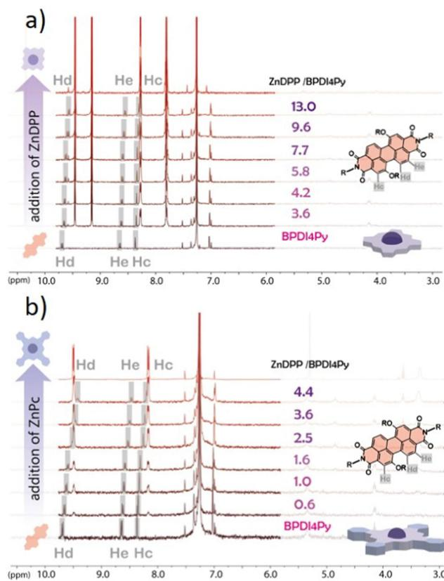
Fig. 5 (a) <sup>1</sup>H NMR spectra in CDCl<sub>3</sub> of a titration of BPDIC7 solution (0.5 mL, 0.055 mM) with increasing amounts of ZnPc (180 μL, 0.13 mM) and (b) ZnDPP (400 μL, 13 mM) in CDCl<sub>3</sub>.
