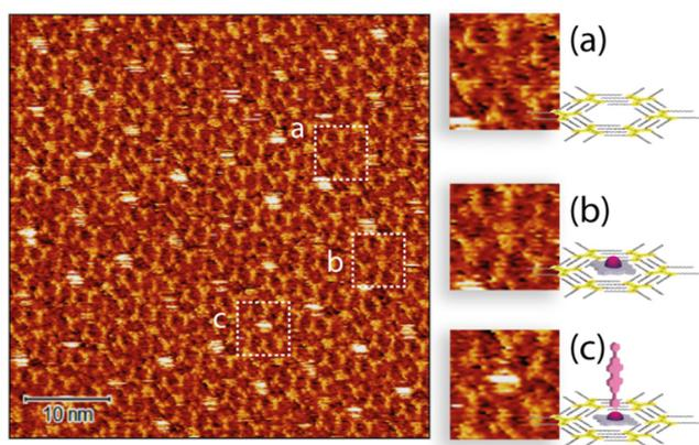
Fig. 6 STM image of a  $50 \times 50 \text{ nm}^2$  area with C10-TSB and the deposited ZnDPP-BPDI4Py dyad on HOPG (bias:  $-0.2 \text{ V}$ , current:  $20 \text{ pA}$ ). Selected areas showing an empty TSB pore (a), the ZnDPP pedestal trapped inside a pore (b) and the ZnDPP-BPDI4Py dyad trapped by the C10-TSB network (c).
