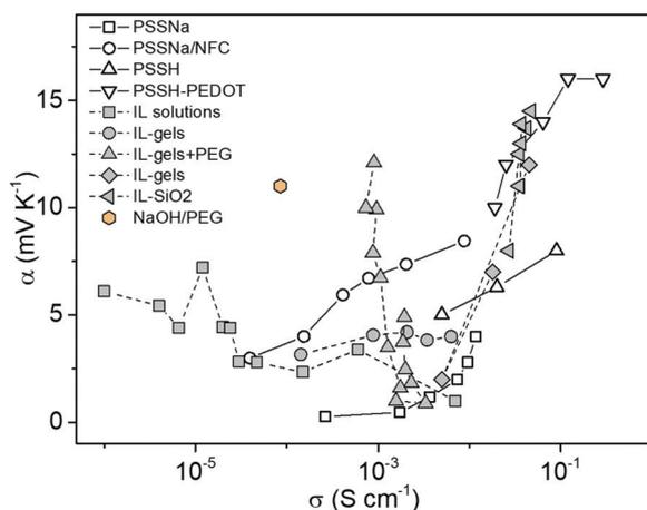
Fig. 1 The distribution of the ionic Seebeck coefficient and conductivity of recently reported electrolytes as thermoelectric materials.<sup>26–28</sup>
