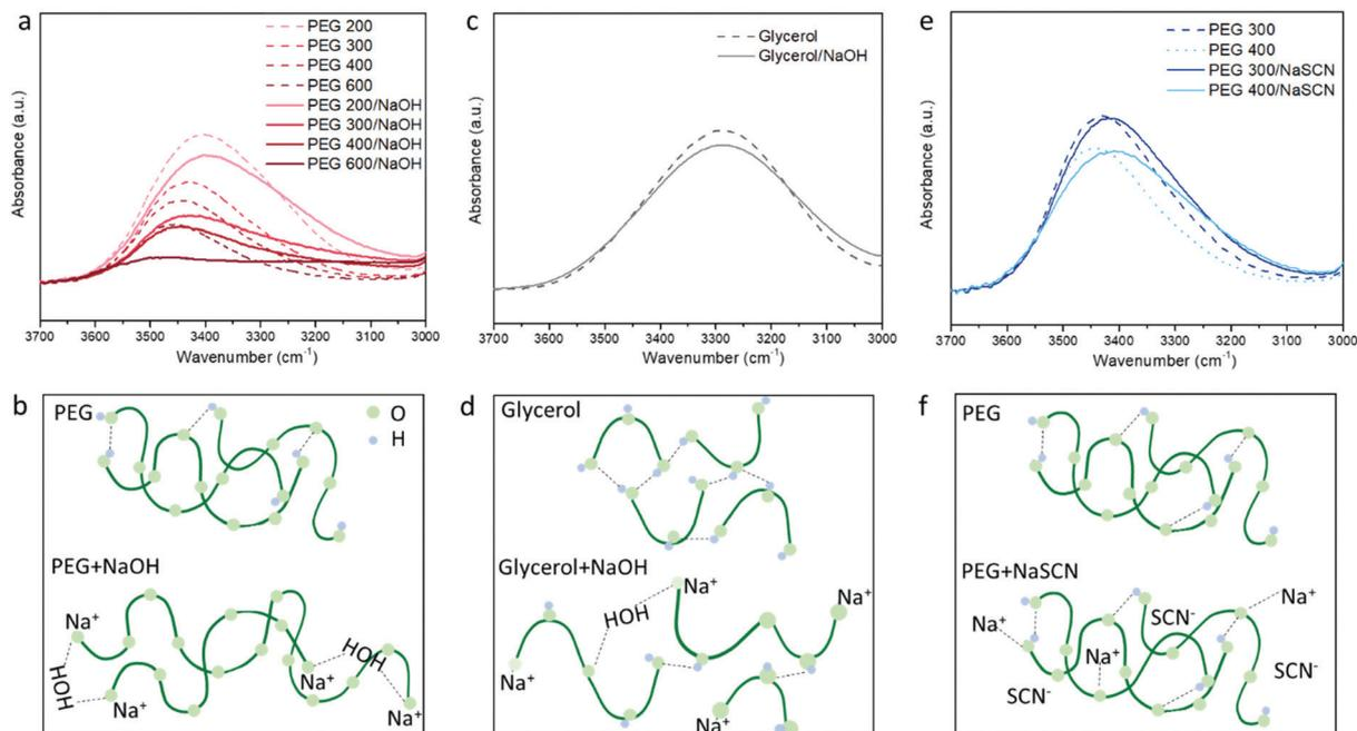
**Fig. 3** The FTIR characterization of different electrolytes in room temperature. (a) The O–H stretching peak and (b) illustration of PEG/NaOH electrolytes. (c) The OH stretching peak and (d) illustration of the glycerol/NaOH electrolyte. (e) The OH stretching peak and (f) illustration of the PEG/NaSCN electrolyte.
