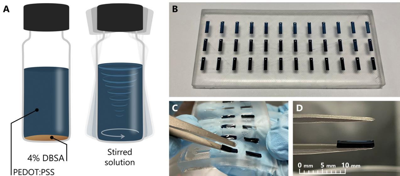
**Fig. 1** The fabrication of PEDOT:PSS hydrogel electrodes. (A) Aqueous PEDOT:PSS suspension is combined with 4% (volume) DBSA, and then stirred using a vortex mixer. (B) The solution is deposited by pipette into wells in a PDMS mould. (C) Once gelation has occurred, the electrodes can be removed from the mould. (D) The electrode (8 mm  $\times$  2 mm  $\times$  1 mm) maintains the shape of the mould.
