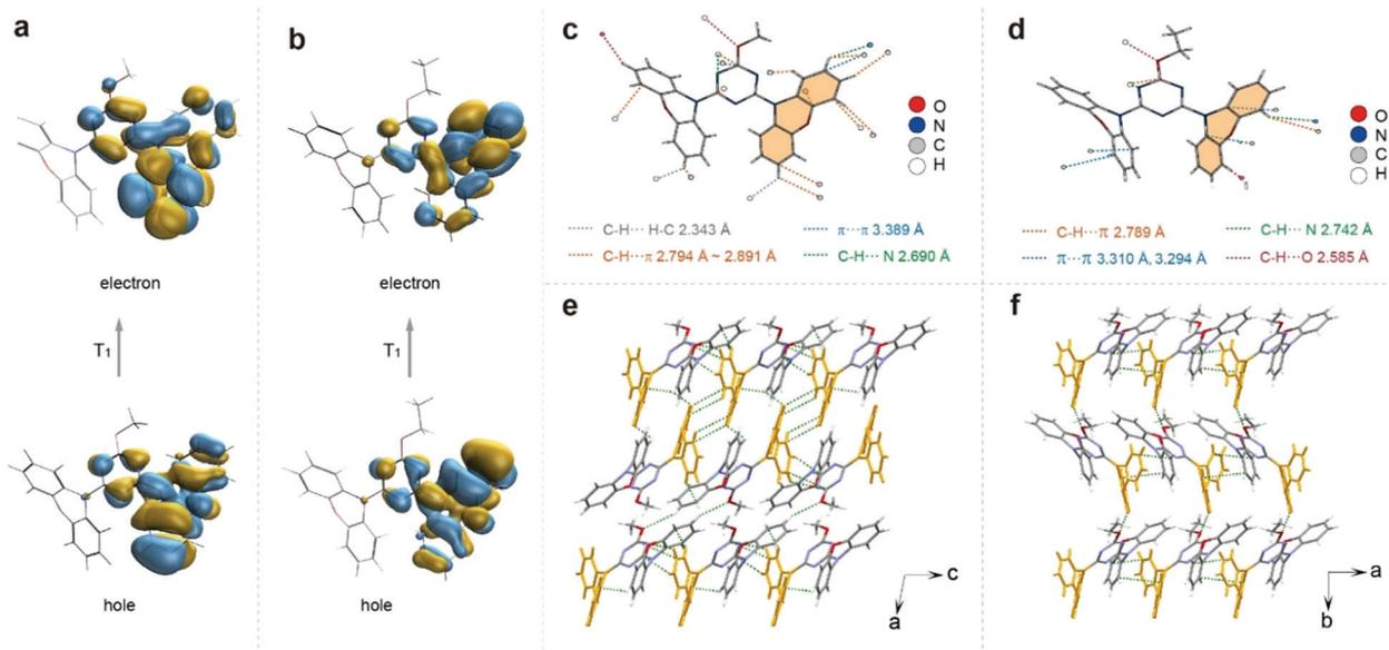
**Fig. 3** Theoretical calculation and crystal analysis of MT and ET molecules. Natural transition orbitals (NTOs) of T<sub>1</sub> states for MT (a) and ET (b) molecules. Intermolecular interactions around one molecule of MT (c) and ET (d) in the crystal state. The packing modes of MT (e) and ET (f) crystals. The yellow labels in e and f represent the triplet chromophore.
