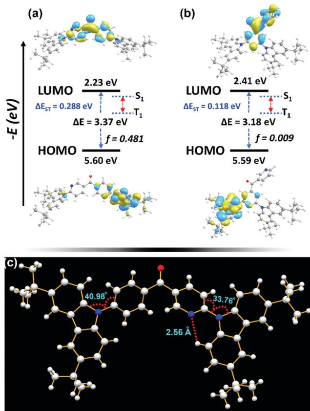
Fig. 1 DFT calculated electron density distributions of the highest occupied molecular orbital (HOMO) and the lowest unoccupied molecular orbital (LUMO) of (a) **3BPpy-pDTC** and (b) **3BPpy-mDTC** at the B3LYP/6-311G(d,p) level. (c) The molecular structure and packing diagram of **3BPpy-pDTC** obtained from single crystal X-ray diffraction (SCXRD) analysis displaying the intramolecular H-bonding interaction and the donor-acceptor dihedral angles.
