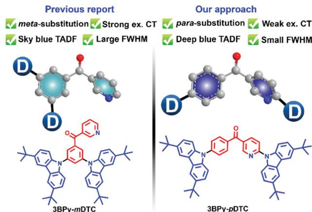
Scheme 1 Molecular design strategy of a blue TADF emitter: a comparative account of the intrinsic ICT interactions of *meta* and *para* substituted donors on the 3BPpy acceptor core. The molecular structures of *meta*-substituted **3BPpy-*m*DTC** and *para*-substituted **3BPpy-*p*DTC** with DTC as the donor units are shown.
