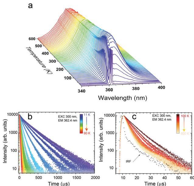
Fig. 4 (a) Normalized (at 362.4 nm) temperature-dependent luminescence spectra of the  $\text{SrB}_4\text{O}_7:\text{Eu}^{2+}$  material, measured in the 11–600 K range upon excitation at 300 nm. Temperature-dependent decay traces of  $\text{Eu}^{2+}$  luminescence, recorded in the range (b) 11–90 K and (c) 100–600 K range.
