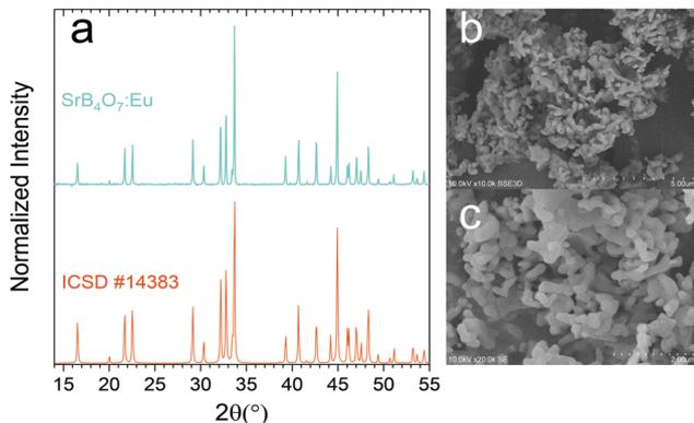
Fig. 2 (a) X-Ray diffraction pattern of  $\text{SrB}_4\text{O}_7$  containing 3% of  $\text{Eu}^{2+}$  and prepared in an air atmosphere. (b) and (c) SEM images of the  $\text{SrB}_4\text{O}_7:\text{Eu}^{2+}$  powder, taken at different magnifications (b -  $5 \mu\text{m}$  scale bar; c -  $2 \mu\text{m}$  scale bar).
