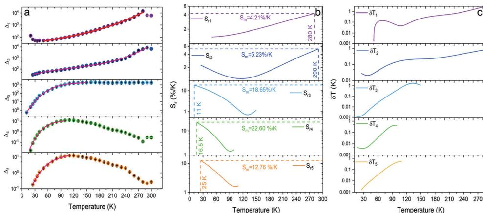
Fig. 7 (a) Thermal evolution of  $\Delta$  parameters for the  $\text{SrB}_4\text{O}_7:\text{Eu}^{2+}$  phosphor, (b) its relative thermal sensitivities, and (c) corresponding temperature uncertainties.
