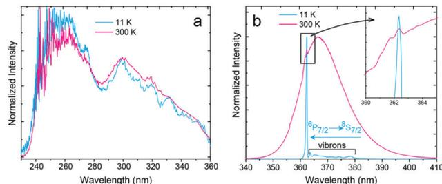
Fig. 3 (a) PLE and PL spectra of  $\text{SrB}_4\text{O}_7:\text{Eu}^{2+}$  microparticles. The PLE spectrum was monitored at 367.2 nm and recorded at 11 and 300 K. (b) PL spectra recorded at 11 K and 300 K excited at 300 nm. In-depth analysis of the ZPL lines and vibronic transitions was presented in ref. 8.
