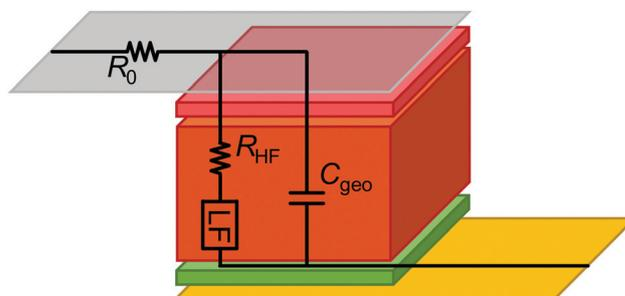
Fig. 6 Schematic with series resistance  $R_0$ , high-frequency resistance  $R_{HF}$ , and a potential LF feature. Grey and yellow rectangles represent the current collectors, and the brown, red and green layers represent the absorber and transport layers, respectively.
