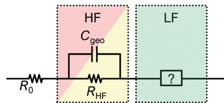
Fig. 8 General structure of the proposed ECM.  $R_0$  accounts for the Ohmic resistance of the contacts and current collectors,  $C_{\text{geo}}$  is the geometrical capacity,  $R_{\text{HF}}$  is the sum of all HF features in the spectrum and the LF-ECM will be detailed below.
