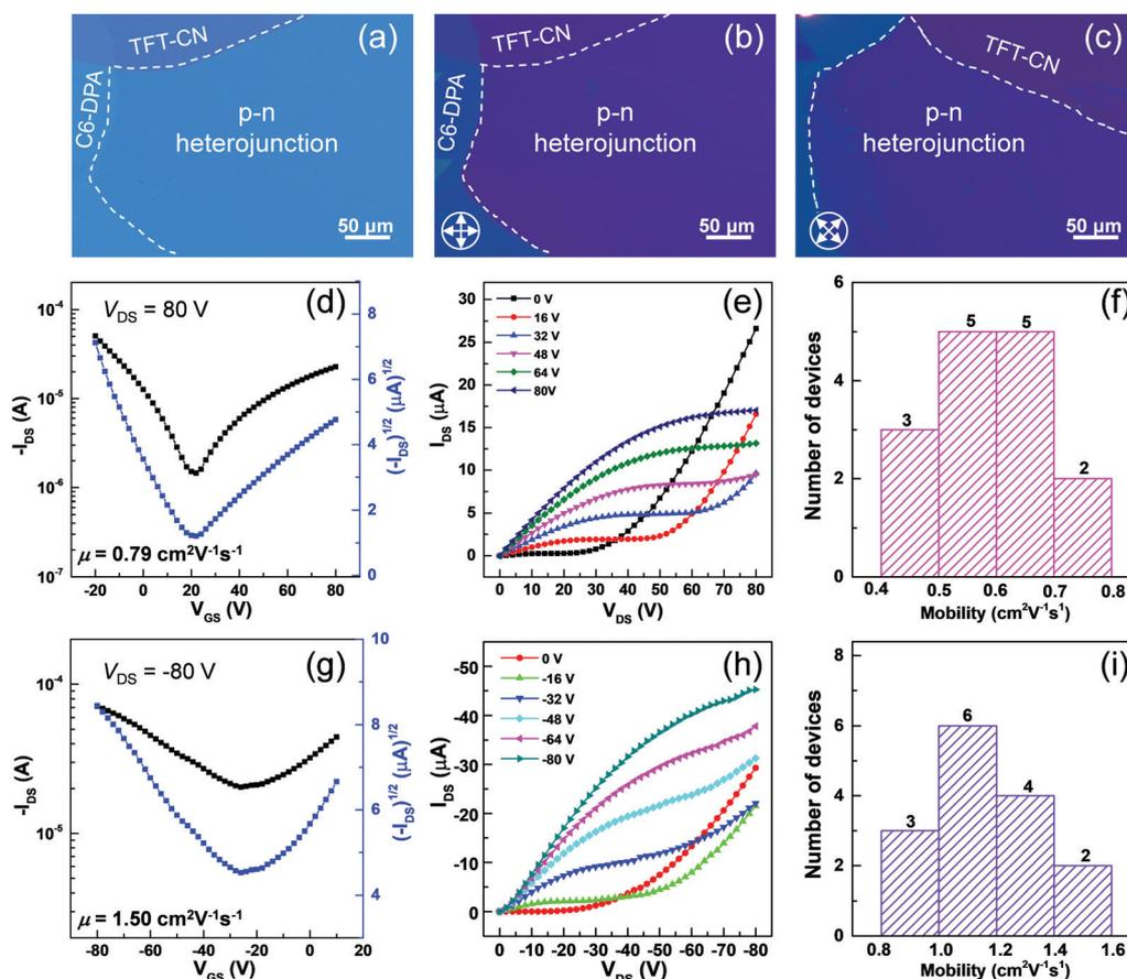
Fig. 4 (a) OM and (b and c) POM images of the p-n heterojunctions. (d) Transfer characteristics, (e) output characteristics, and (f) the mobility distribution at  $V_{DS} = 80$  V. (g) Transfer characteristics, (h) output characteristics, and (i) the mobility distribution at  $V_{DS} = -80$  V.
