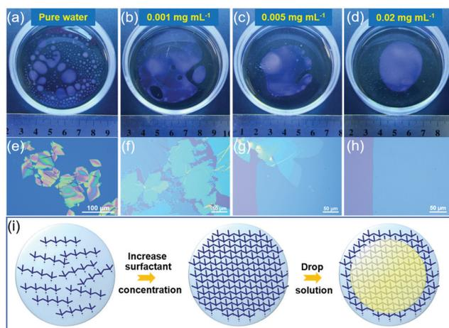
**Fig. 1** The spreading of a toluene solution of C6-DPA on water without the surfactant and with different concentrations of the surfactant. The concentrations of the surfactant were (a) 0, (b)  $0.001 \text{ mg mL}^{-1}$ , (c)  $0.005 \text{ mg mL}^{-1}$  and (d)  $0.02 \text{ mg mL}^{-1}$ . (e–h) Corresponding OM images of the C6-DPA 2DMCs grown on the water substrate. (i) Schematic diagram of the principle of the STAS strategy.
