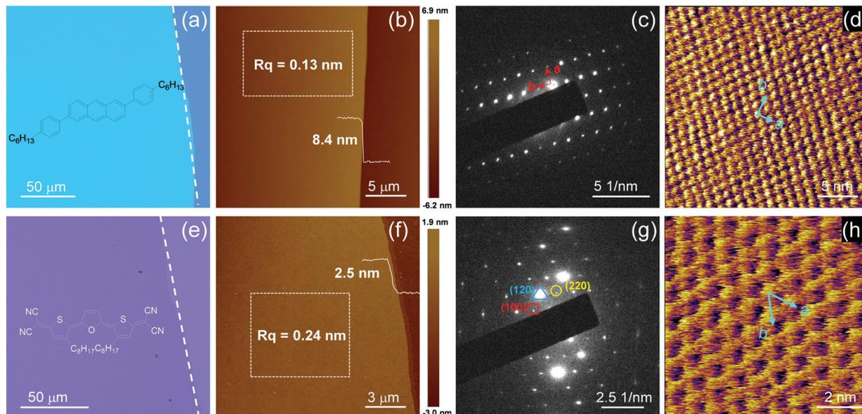
Fig. 2 (a) OM image, (b) AFM image, (c) SAED pattern and (d) HRAFM image of a C6-DPA 2DMC. (e) OM image, (f) AFM image, (g) SAED pattern and (h) HRAFM image of a TFT-CN 2DMC.
