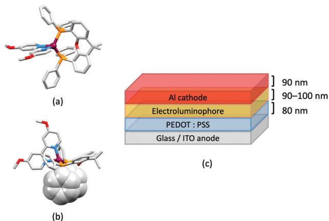
Fig. 9 (a) Structure of the cation in  $[\text{Cu}(\text{xantphos})(4,4'\text{-(MeO)}_2\text{bpy})][\text{BF}_4]$  (CSD refcode VANYOB), and (b) illustration of the  $\pi$ -stacking interaction between adjacent  $\text{PPh}_2$  units. H atoms are omitted for clarity. (c) Architecture of the LECs containing the Cu-iTMCs  $[\text{Cu}(\text{xantphos})(4,4'\text{-R}_2\text{bpy})][\text{BF}_4]$  with  $\text{R} = \text{MeO}, \text{Me}, \text{H}$ . LECs were driven using a pulsed current.
