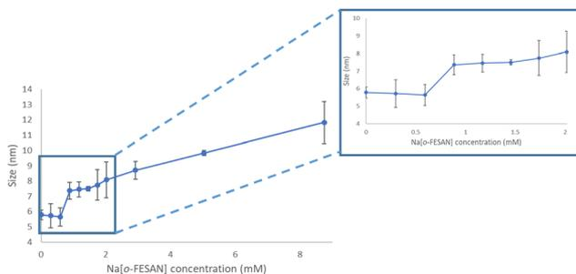
Fig. 5 Graphical representation of the hydrodynamic diameter (nm) of the DMEM + 10% FBS culture medium measured by DLS versus increasing concentrations of  $\text{Na}[o\text{-FESAN}]$  in water in the concentration range from 0 to 9 mM.
