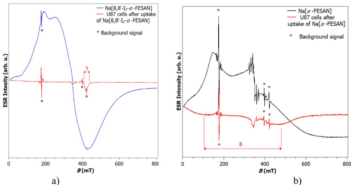
**Fig. 1** (a) Spectra of Na[8,8'-I<sub>2</sub>-o-FESAN] in powder, U87 cells after uptake of Na[8,8'-I<sub>2</sub>-o-FESAN]. The *g* factor indicated by number 5 is 1.7. (b) Spectra of Na[o-FESAN] in powder and U87 cells after uptake of Na[o-FESAN]. The *g* factor indicated by number 6 is approximately 2.
