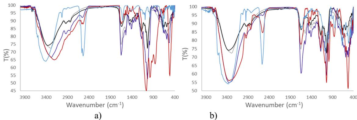
Fig. 3 (a) IR spectra of 2 mM Na[*o*-FESAN] in aqueous solution (blue), in DMEM (without phenol red) (red), and in DMEM + 10% FBS (purple). (b) IR spectra of 2 mM Na[8,8'-I<sub>2</sub>-*o*-FESAN] in aqueous solution (blue), in DMEM (red), and in DMEM + 10% FBS (purple). As a control: IR spectra of DMEM (black) and DMEM + 10% FBS (grey).
