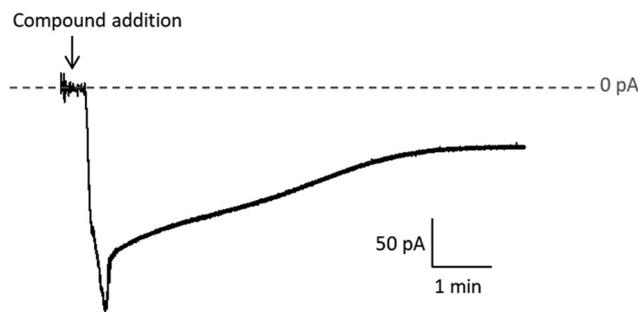
Fig. 6 Sample current recording after Na[*o*-FESAN] addition to the feeding side of the chamber. The stripping side was electrically grounded. Negative current implies that the [*o*-FESAN]<sup>-</sup> anion crosses the membrane.
