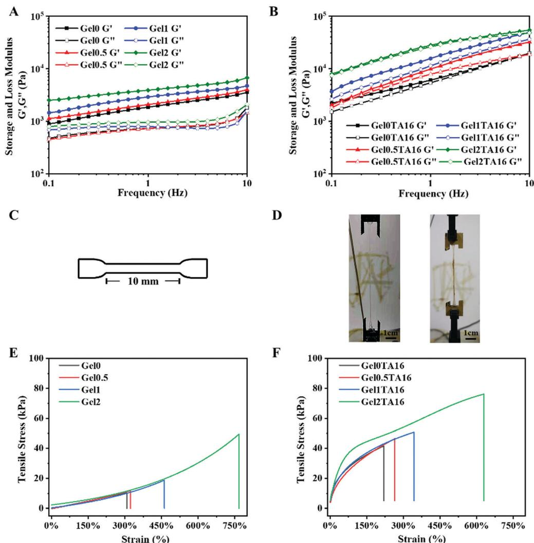
Fig. 3 The mechanical properties of the hydrogels: the rheological properties of (A) gel and (B) gel/TA hydrogels; (C) a diagram of a tensile test strip; (D) images of tensile testing; and the tensile stress data for (E) gel and (F) gel/TA hydrogels.
