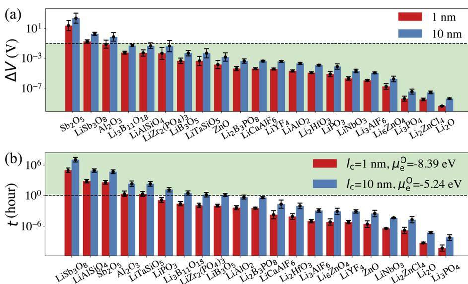
Fig. 5 (a) Calculated overpotentials ( $\Delta V$ ) for a current density of  $0.044 \text{ mA cm}^{-2}$  across room temperature cathode coatings of  $l_c = 1$  and  $10 \text{ nm}$ . The dashed line represents  $\Delta V = 0.1 \text{ V}$ . (b) Calculated  $\text{O}^{2-}$  diffusion time  $t$  in the selected compounds assuming a  $r = 1 \mu\text{m}$  primary particle and an  $l_s = 2 \text{ nm}$  surface rocksalt phase. The dashed line represents  $t = 1 \text{ h}$ .
