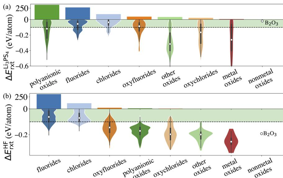
Fig. 3 Distribution of the reaction energy  $\Delta E_{\text{rxt}}$  with  $\text{Li}_3\text{PS}_4$  (a) and HF (b) for each category that pass chemical stability with the cathodes descriptor. The horizontal dash lines represent the limits of the descriptors. The histograms in (a) and (b) illustrate the numbers of compounds for each category that pass the descriptors.
