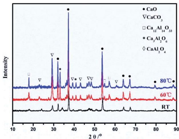
Fig. 6 XRD patterns of the Ca–Al mixed oxides ( $\text{Ca}^{2+}/\text{Al}^{3+} = 3$ ) synthesised at room temperature (RT), 60 °C and 80 °C. Reprinted with permission<sup>66</sup> copyright 2021 Elsevier.
