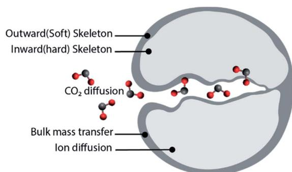
Fig. 2 The pore skeleton model for CO<sub>2</sub> and ion diffusion. Illustrated according to the finding presented in ref. 51.
