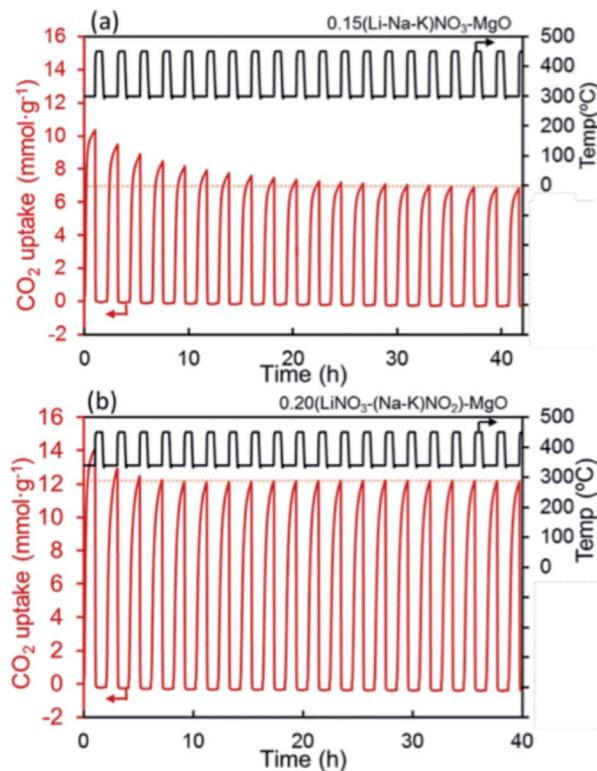
Fig. 8 CO<sub>2</sub> capture capacity of promoted MgO by alkali metal nitrates ((Li–Na–K)NO<sub>3</sub>) and nitrate/nitrite (LiNO<sub>3</sub>–(Na–K)NO<sub>2</sub>) salt. Reprinted with permission<sup>86</sup> copyright 2021 American Chemical Society.
