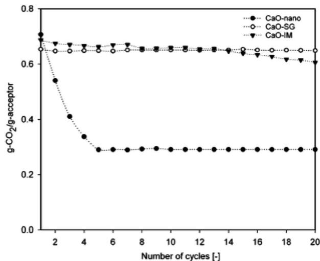
Fig. 5 CO<sub>2</sub> capture capacity of nano-CaO by sol–gel and wet impregnation methods. Reprinted with permission from ref. 59. Copyright 2021 American Chemical Society.
