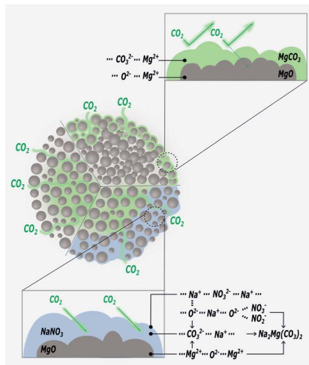
Fig. 7 The role of the MgO sorbent with nitrate salts for improving CO<sub>2</sub> capture capacity.
