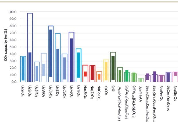
Fig. 11 Theoretical and experimental CO<sub>2</sub> uptake capacities of various Li-, Na-, K-, Sr- and Ba- based CO<sub>2</sub> sorbents. The hollow bars represent the stoichiometric capture capacities, whereas the solid bars represent the range of experimentally measured CO<sub>2</sub> uptakes. The sorbents are classified according to the chemical composition of the active components, *i.e.* excluding the formulation of the support.
