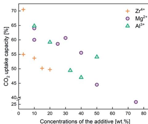
Fig. 4 CO<sub>2</sub> capture capacity of CaO based sorbents stabilised by the three different typical sintering-resistant, oxidic additives containing Zr<sup>4+</sup>, Al<sup>3+</sup>, and Mg<sup>2+</sup>. The effect of these additives on the cyclic stability of CaO sorbents is summarised in Table 2.
