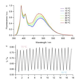
Fig. 3 (a) Temperature-dependent emission of  $4^{\rm Py}$  in MeCN (2.6  $\times$   $10^{-6}$  M), normalised to monomer emission peak and (b)  $I_{\rm E}/I_{\rm M}$  ratio during thermal cycling (10  $\rightleftharpoons$  70 °C).
