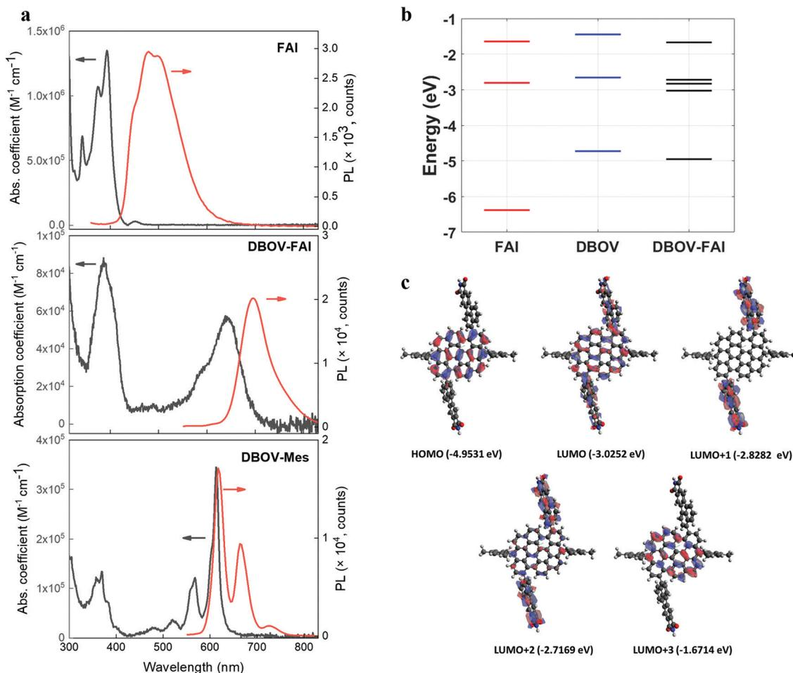
**Fig. 2** (a) Absorption (expressed as molar absorption coefficient) and photoluminescence spectra of FAI (compound **2** in Fig. 1a), DBOV-FAI and DBOV-Mes recorded in toluene at  $10^{-5}$  M (b). For obtaining the photoluminescence spectra, the molecules were excited at 321 nm, 525 nm and 519 nm for FAI, DBOV-FAI and DBOV-Mes, respectively. (b) Energy levels of the three molecules calculated by means of the DFT method. (c) HOMO–LUMO distribution of DBOV-FAI based on DFT calculations.
