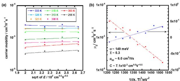
Fig. 8 (a) Hole mobilities plotted for the square root of the electric field at various temperatures in the N\* phase of the compounds **1–3** mixture (low temperature region). (b) Plots of zero-field mobility  $\mu_0$  and  $\beta$  as a function of the square of  $1/k_B T$  in the N\* phase of the LC mixture (low temperature region).
