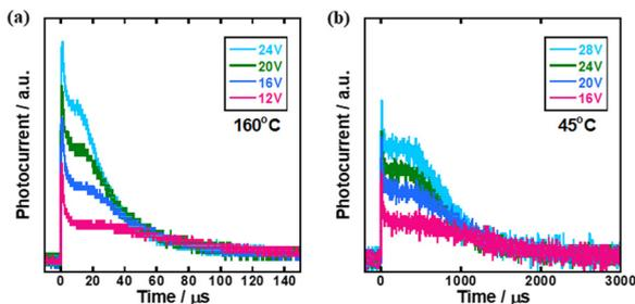
Fig. 6 Transient photocurrent curves for holes (a) in the N\* phase of the mixture of compounds **1–3** at 160 °C and (b) in the glassy N\* phase at 45 °C. The sample thickness was 4 μm and the wavelength of excitation light was 356 nm.
