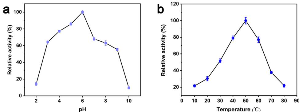
Fig. 5 Dependence of the Au/UiO-66 peroxidase-like activity on reaction conditions: (a) pH and (b) temperature.
