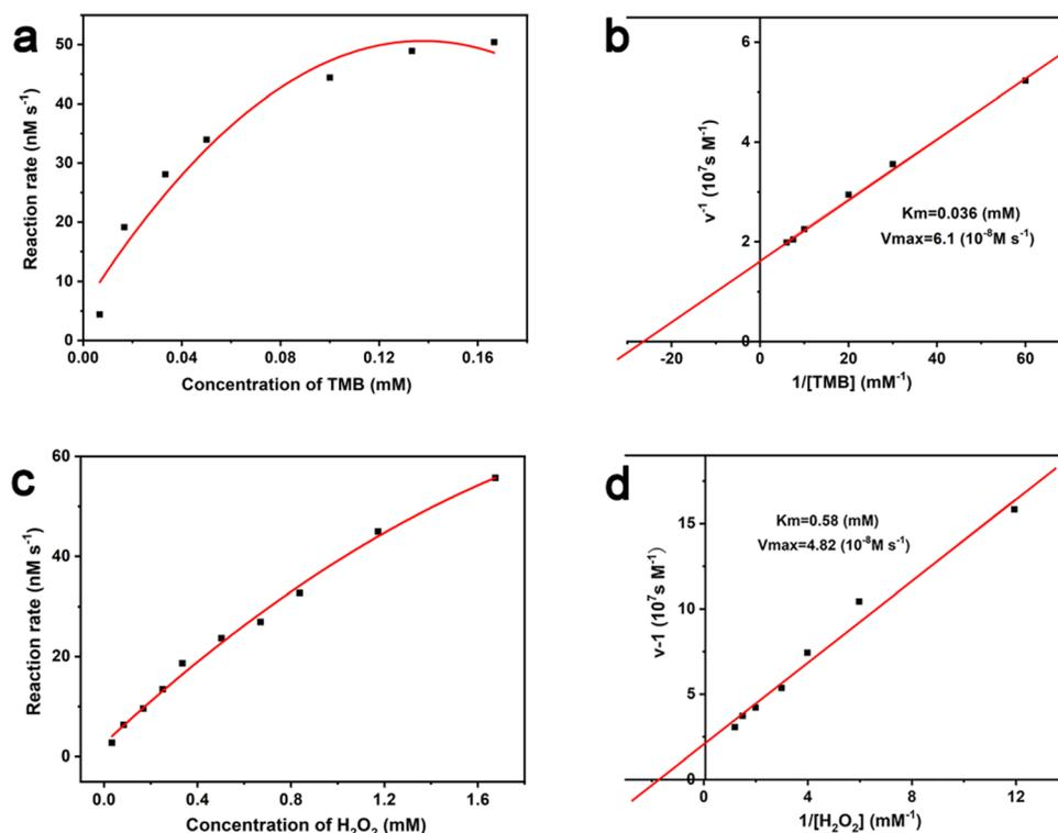
Fig. 6 (a) Effect of TMB concentration on the Au/Uio-66 catalytic oxidation TMB reaction rate. (b) The corresponding double reciprocal graph of (a). (c) The effect of H<sub>2</sub>O<sub>2</sub> concentration on the reaction rate of Au/Uio-66 catalyzed TMB oxidation. (d) The corresponding double reciprocal graph of (c).
