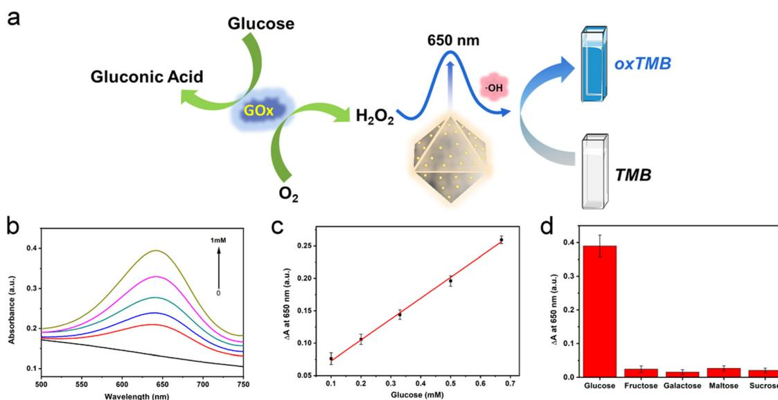
Fig. 7 (a) A schematic diagram of detection for glucose using Au/UiO-66. (b) Evolution of UV-Vis absorption spectra with increasing glucose concentration. (c) The standard curve of  $\Delta A$  at 650 nm with increasing glucose concentration. (d) Selectivity of the glucose detection method.
