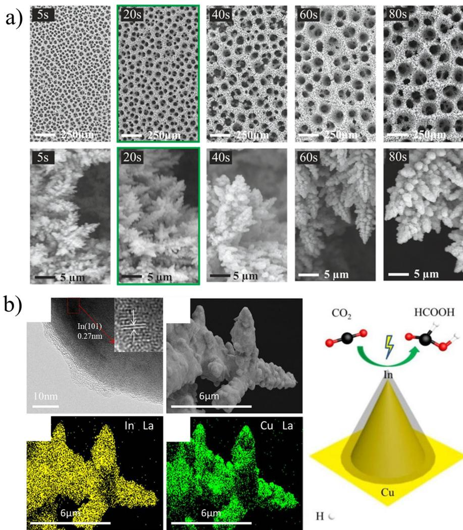
Fig. 7 (a) SEM micrographs showing the changes of surface pore size and dendrite size with deposition time. Reproduced with permission.<sup>46</sup> Copyright 2021, American Chemical Society. (b) HRTEM images of the Cu–In–30 catalyst, SEM image of the Cu–In–30 catalyst, and the corresponding EDX elemental maps. Reproduced with permission.<sup>47</sup> Copyright 2021, American Chemical Society.
