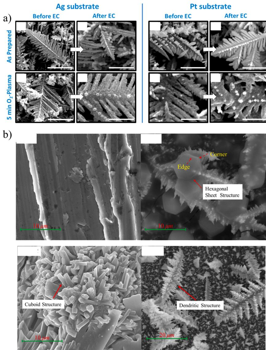
Fig. 3 (a) Scanning electron microscopy (SEM) images of catalysts prepared under different conditions before and after the CDRR reaction. Reproduced with permission.<sup>24</sup> Copyright 2019, American Chemical Society. (b) SEM images of copper and deposits of Bi obtained by different electrodeposition methods: constant potential, CP; direct current, DC; and pulse current, PC. Reproduced with permission.<sup>26</sup> Copyright 2021, Elsevier.
