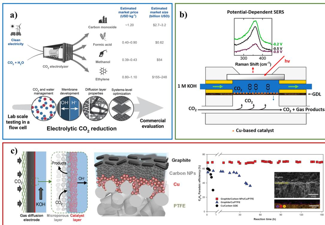
Fig. 13 (a) An overview of the market for CDRR products and the application of flow cell. Reproduced with permission.<sup>82</sup> Copyright 2018, American Chemical Society. (b) Schematic diagram of the flow tank structure. Reproduced with permission.<sup>40</sup> Copyright 2019, American Chemical Society. (c) Schematic diagrams of flow cell cathode and the catalytic performance. Reproduced with permission.<sup>81</sup> Copyright 2018, American Association for the Advancement of Science.
