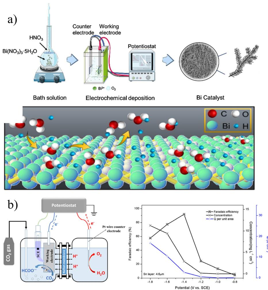
Fig. 2 (a) Schematic diagram of the two-electrode system for constant current deposition of bismuth electrodes. Reproduced with permission.<sup>22</sup> Copyright 2021, Elsevier. (b) Schematic diagram of electrocatalytic reduction of carbon dioxide in a three-electrode system and a summary of its performance. Reproduced with permission.<sup>23</sup> Copyright 2016, Elsevier.
