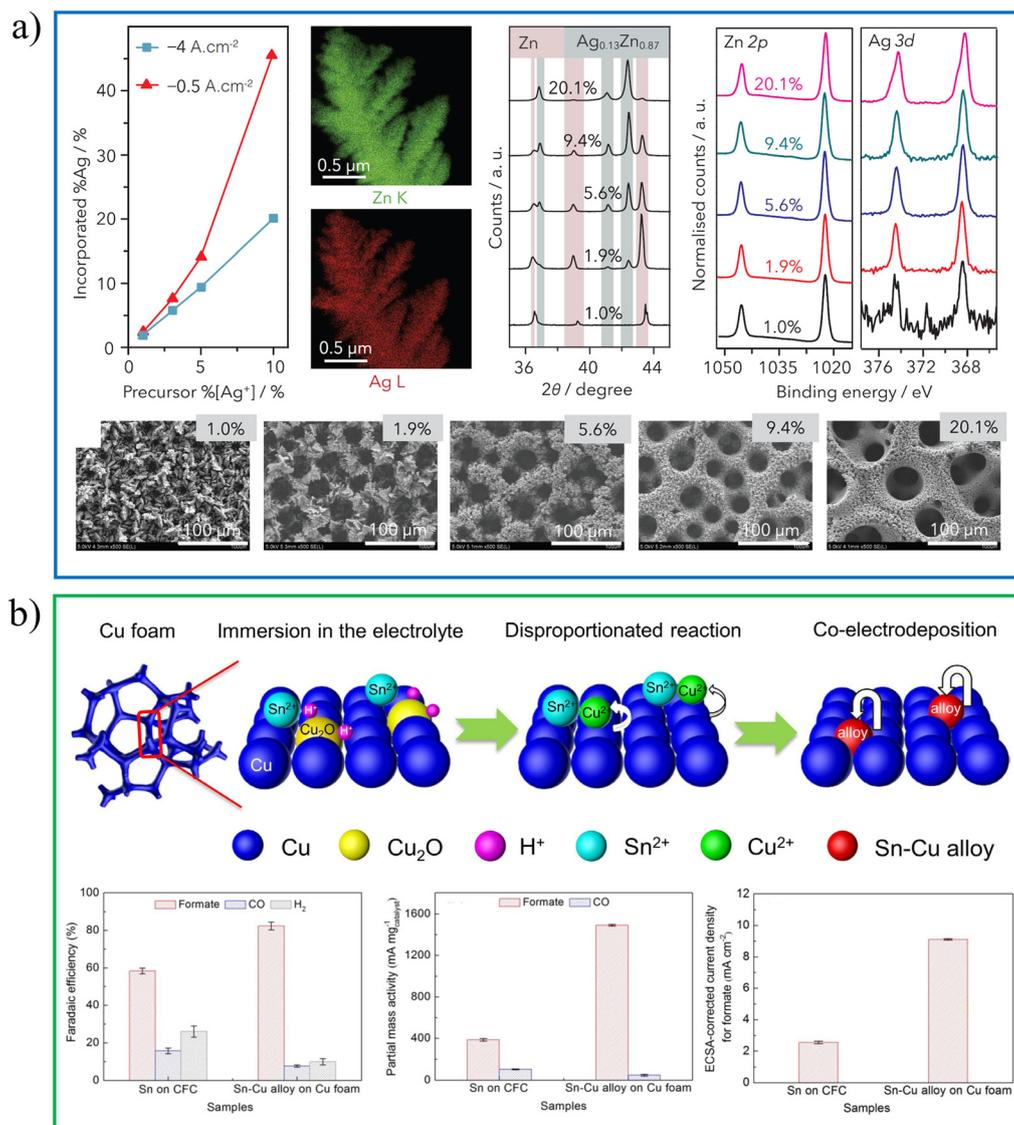
Fig. 4 (a) Ag-Zn alloy growth and characterization. Reproduced with permission.<sup>27</sup> Copyright 2020, Elsevier Inc. (b) Schematic diagram of SnCu alloy preparation and catalytic performance. Reproduced with permission.<sup>28</sup> Copyright 2020, Elsevier.
