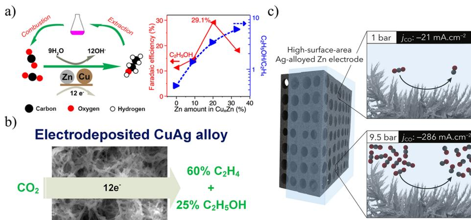
Fig. 10 (a) Schematic diagram of ethanol production from CuZn alloy. Reproduced with permission.<sup>58</sup> Copyright 2016, American Chemical Society. (b) Schematic diagram of the production of C2 products from CuAg alloys. Reproduced with permission.<sup>17</sup> Copyright 2018, American Chemical Society. (c) Schematic diagram of efficient CO production from AgZn alloy. Reproduced with permission.<sup>27</sup> Copyright 2019, Elsevier Inc.
