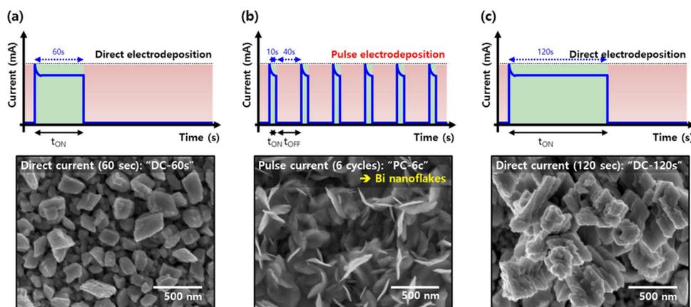
Fig. 5 Current curves and the corresponding SEM images of direct electrodeposition and pulse electrodeposition. Reproduced with permission.<sup>29</sup> Copyright 2017, Elsevier.
