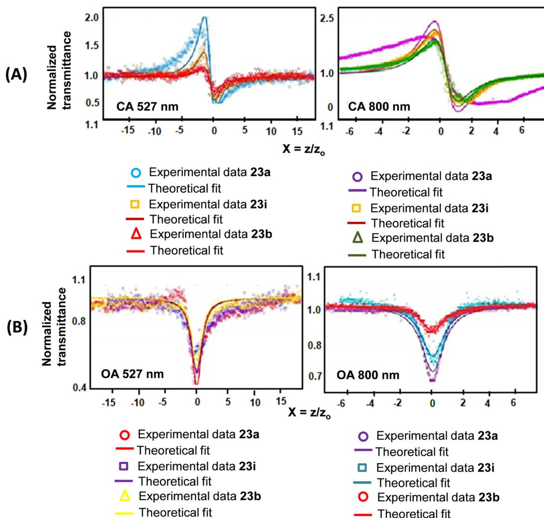
**Fig. 18** Z-scan traces of **23a**, **23i** and **23b** in DCM under (A) closed aperture (CA) and (B) open aperture (OA) conditions at (i) 527 nm and at (ii) 800 nm. Reproduced with permission from ref. 40. Copyright 2016, The Royal Society of Chemistry.
