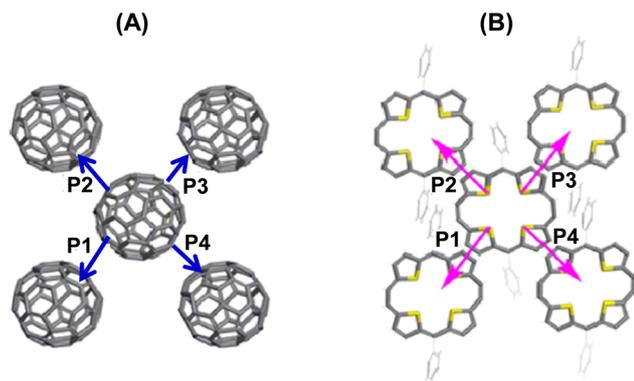
Fig. 16 Charge hopping pathways of the (A) acceptor ( $C_{60}$ ) and (B) donor (**22a**) components in the individual molecular layers. Reproduced with permission from ref. 32. Copyright 2013, The American Chemical Society.
