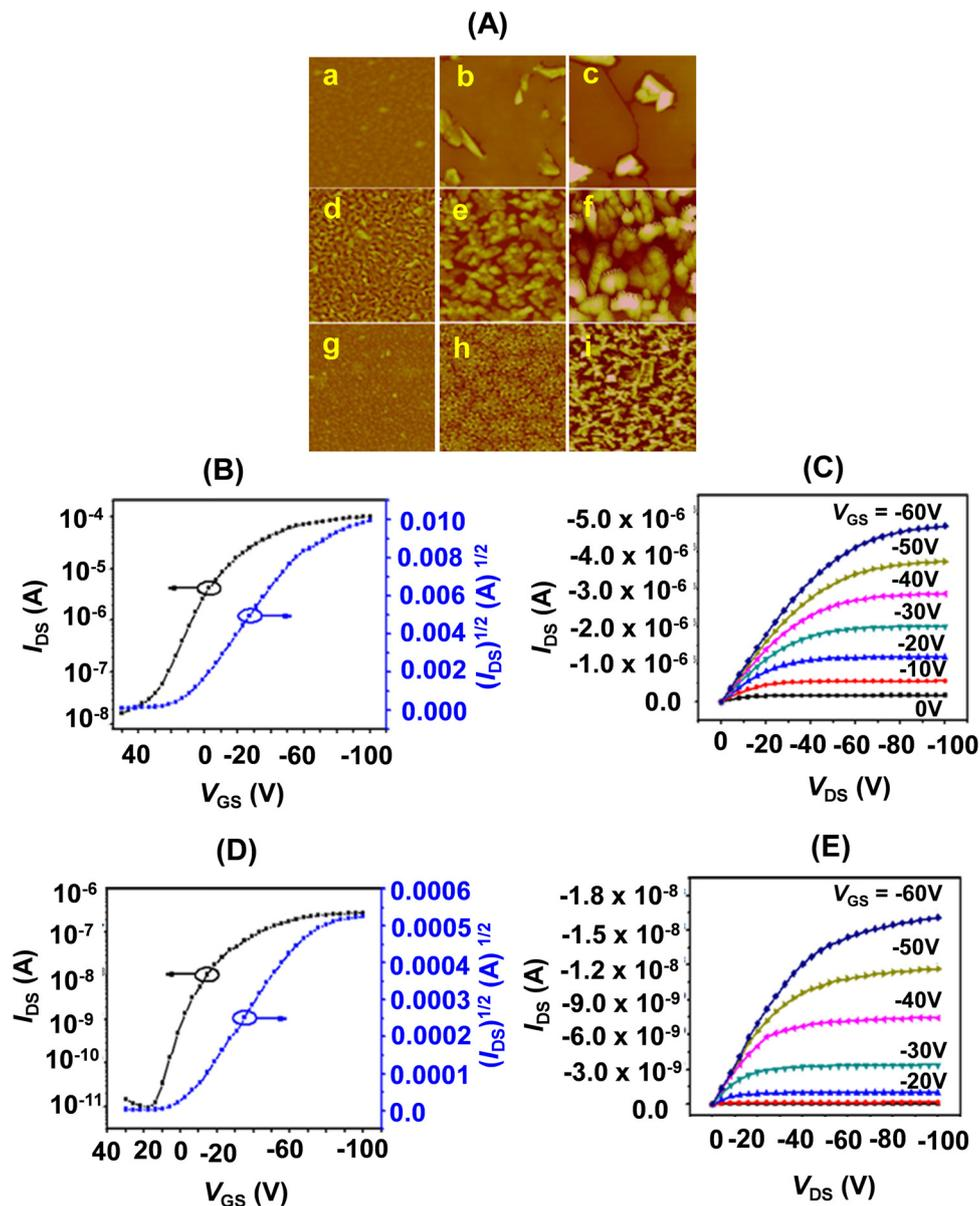
Fig. 9 (A) AFM images ( $5 \times 5 \mu\text{m}$ ) of 50 nm thick films of **22f–h**, (a, d and g)  $T_s = 25^\circ\text{C}$ ; (b, e and h)  $T_s = 60^\circ\text{C}$ ; (c, f and i)  $T_s = 100^\circ\text{C}$ . (B/D) Transfer and (C/E) output characteristics of the thin film OFET devices of **22f/22g** (deposited on OTS treated  $\text{SiO}_2/\text{Si}$  substrate ( $T_s = 25^\circ\text{C}$ )). Reproduced with permission from ref. 19. Copyright 2014, The Royal Society of Chemistry.
