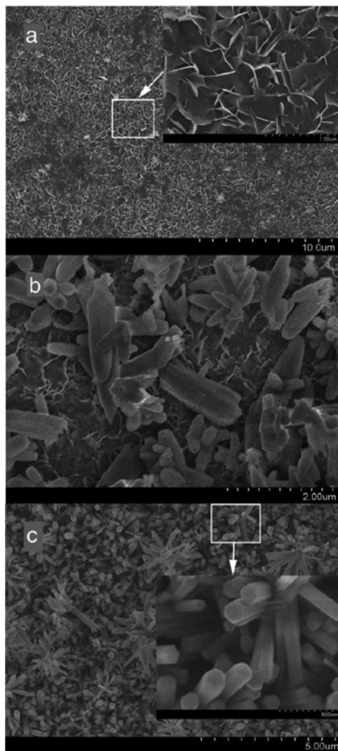
Fig. 3 Microstructural modifications of the coating electrodeposited at  $-1.8$  V over various time intervals of (a) 10 min, (b) 20 min and (c) 60 min. Adapted from ref. 77 with permission from Elsevier.
