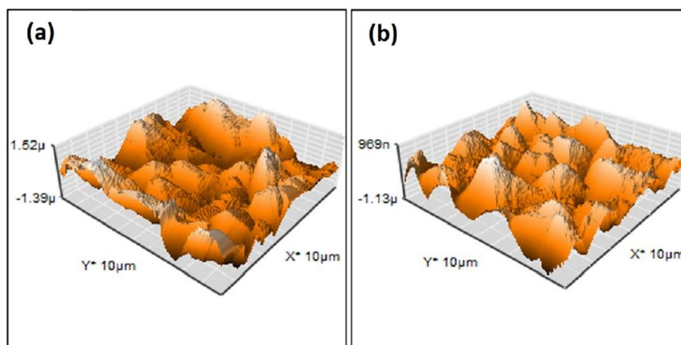
Fig. 5 AFM surface profile of HAP deposited *via* pulse electrodeposition in (a) the absence of ultrasonic irradiation and (b) at 60 W ultrasonic power. Adapted from ref. 98 with permission from Elsevier.
