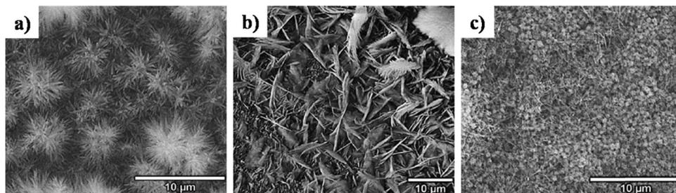
Fig. 9 FESEM of HAP crystals deposited *via* the simultaneous precipitation–electrodeposition technique with dropwise addition of (a) P precursor, (b) Ca precursor and (c) Ca + P precursor. Reproduced from ref. 120 with permission from Elsevier.
