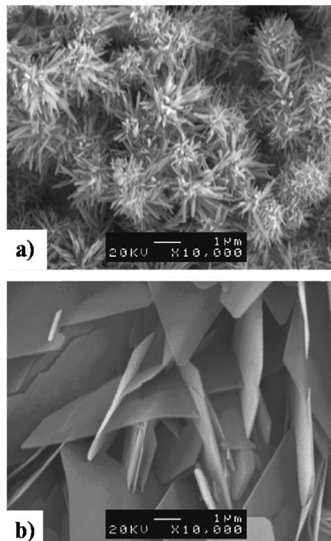
Fig. 15 SEM depicting the formation of (a) needle-like HAp in a  $\text{N}_2$  atmosphere and (b) plate-like HAp in a  $\text{CO}_2$  atmosphere electrodeposited under galvanostatic conditions. Adapted from ref. 152 with permission from Elsevier.
