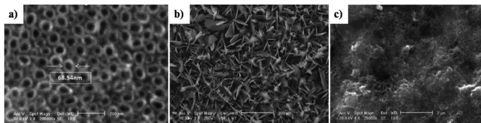
Fig. 16 SEM images depicting the microstructural variation in HAP coating electrodeposited over TiO<sub>2</sub> NT and –COOH functionalized MWCNT/TiO<sub>2</sub> NT substrates: (a) TiO<sub>2</sub> NTs, (b) HAP/TiO<sub>2</sub> NT nanocomposite and (c) HAP/MWCNT/TiO<sub>2</sub> NT nanocomposite. Adapted and rearranged from ref. 160 with permission from Elsevier.
