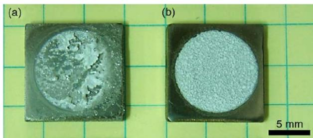
Fig. 14 The enhanced adhesive strength displayed by electrodeposited HAp specimens onto  $\text{Ti}_6\text{Al}_4\text{V}$  at (a) ambient pressure and (b) 80 Torr reduced pressure. Adapted from ref. 150 with permission from Elsevier.
