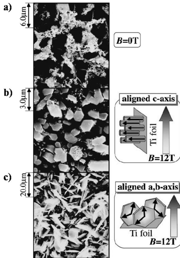
Fig. 11 SEM images of HAP electrodeposited via the heat substrate method over Ti foil under a magnetic field strength of (a)  $B = 0$  T, (b)  $B = 12$  T ( $B \perp j$ ) and (c)  $B = 12$  T ( $B \parallel j$ ). Reproduced from ref. 124 with permission from The Japan Institute of Metals and Materials.
