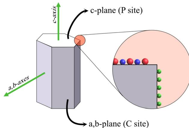
**Fig. 1** Schematic illustration of the hexagonal HAp crystal system with the  $\text{PO}_4^{3-}$  and  $\text{OH}^-$  groups (in red and blue respectively) occupying the  $c$ -plane and  $\text{Ca}^{2+}$  (green sphere) populating the  $a,b$ -plane.
