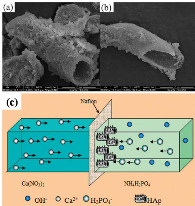
Fig. 19 (a and b) SEM of tubular shaped HAp synthesized *via* the cation exchange membrane-assisted electrodeposition technique and (c) the schematic illustration of the formation of tubular HAp. Images (a) and (b) adapted from ref. 163 and image (c) reproduced from ref. 164 with permission from Royal Society of Chemistry.
