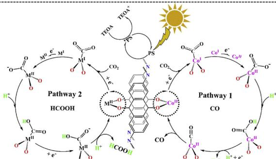
Fig. 7 Synthesis and metallization process of DQTP COF and DATP COF and proposed mechanism for the photocatalytic reduction of CO<sub>2</sub> with DQTP-COF-M (M = Zn, Ni, and Co). Adapted from ref. 107. © 2019 Elsevier B.V. All rights reserved.
