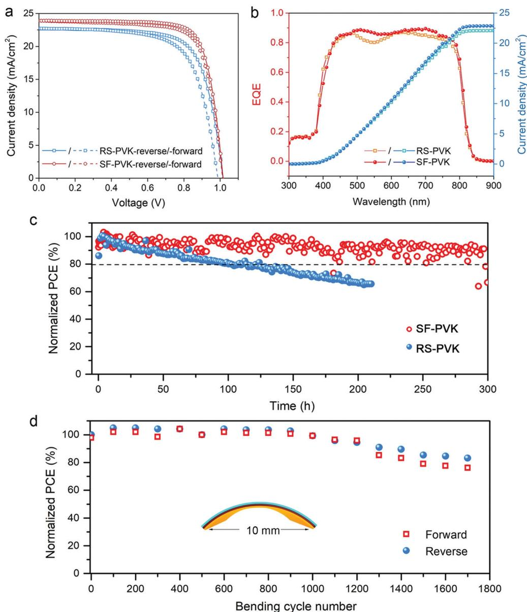
**Fig. 4** (a) Representative  $J-V$  curves of the PSCs made of SF-PVK and RS-PVK with forward and reverse scans. (b) Corresponding EQE spectra of the F-PSCs. (c) Operational stability of un-encapsulated F-PSCs with varying structures measured at a fixed bias near the maximum power point (MPP) under continuous illumination. (d) The PCEs of SF-PSCs as a function of bending cycles.
