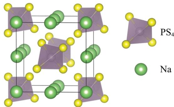
Fig. 3 Schematic depicting the crystal structure of pristine  $t\text{-Na}_3\text{PS}_4$ .<sup>146</sup>
