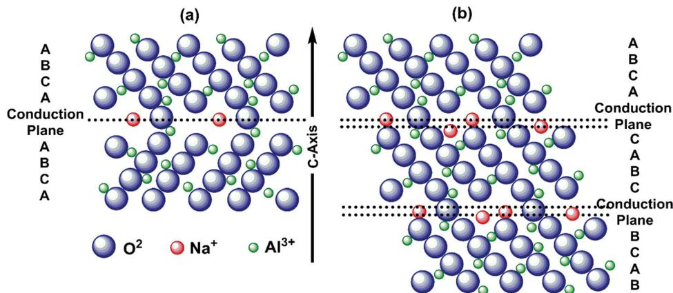
Fig. 10 Schematic representation showing the sequence of stacking and sodium ion conduction plane for (a)  $\beta$ -alumina and (b)  $\beta''$ -alumina.
