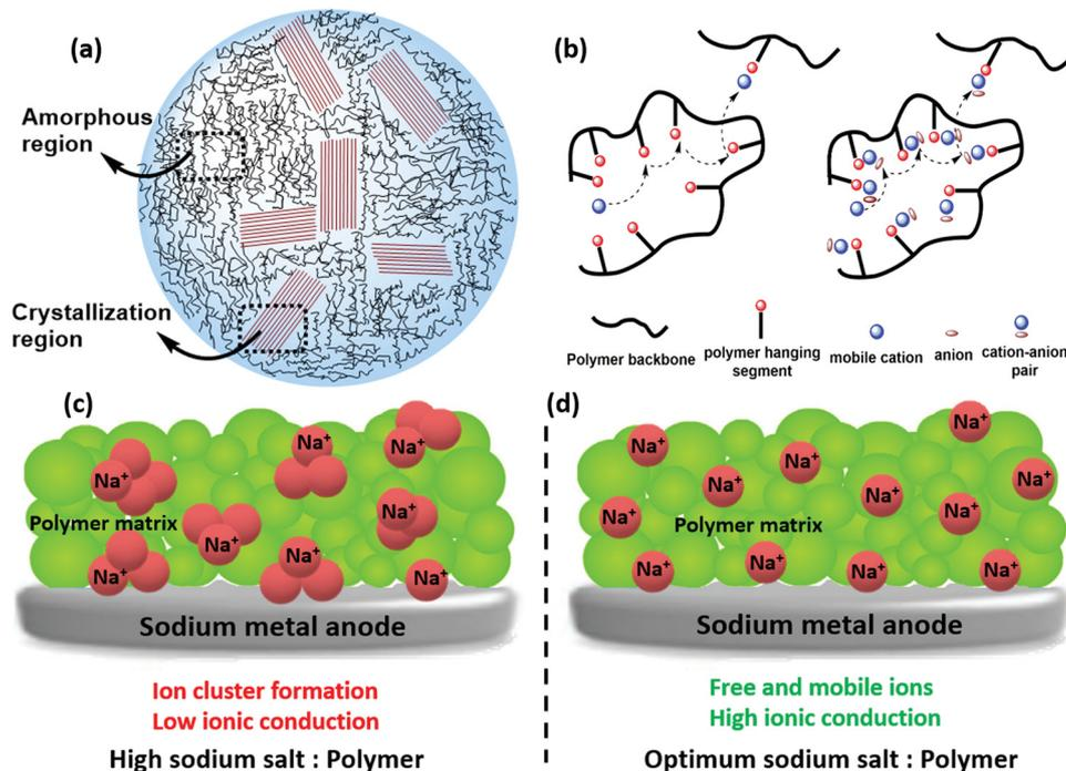
**Fig. 13** Schematic representation showing the mechanism of ionic conduction in solid polymer electrolyte (SPE). (a) Microstructure of a polymer (b) ionic transport at lower salt concentration, (c and d) schematic representation of the effect of sodium salt concentration in the solid polymer matrix. A high sodium salt concentration causes ion clusters that lower ionic mobility, while the optimum level of sodium salt helps in better ion dispersion producing high ionic conduction.
