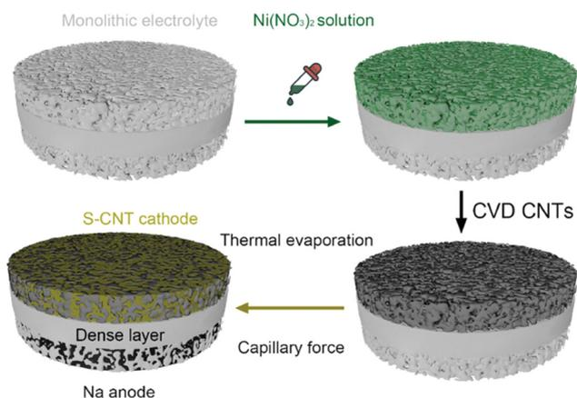
**Fig. 9** Schematic representation of depositing nickel nitrate ( $\text{Ni}(\text{NO}_3)_2$ ) solution and chemical vapor deposited CNT over monolithic electrolyte with the cell architecture of a solid-state RT Na-S battery.<sup>129</sup>
