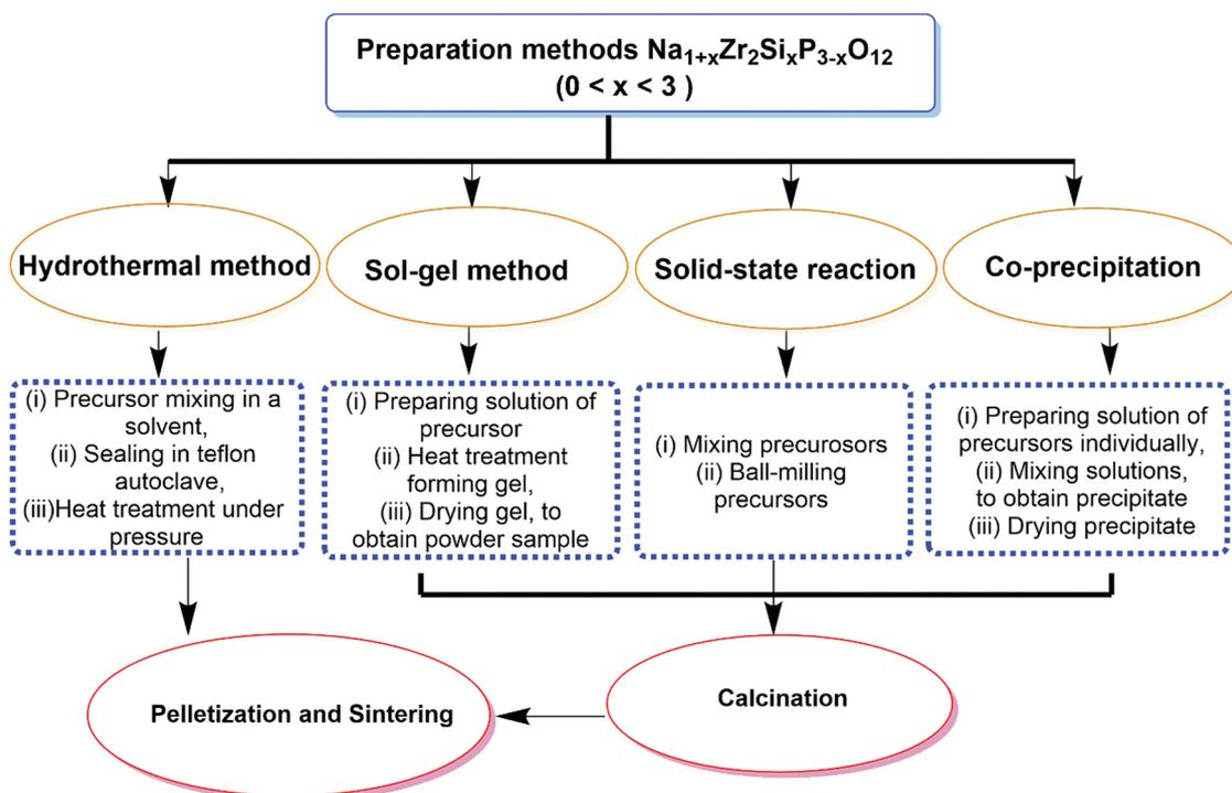
Fig. 6 Flow chart depicting various preparation methods for  $\text{Na}_{1+x}\text{Zr}_2\text{Si}_x\text{P}_{3-x}\text{O}_{12}$ , where the value of  $x$  is given by  $0 \leq x \leq 3$  (NZSP<sub>*x*</sub>).
