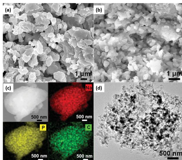
Fig. 4 Morphological analysis and elemental mapping of the  $\text{Na}_3\text{PS}_4$  solid electrolyte and nanocomposite cathode. (a and b) Scanning electron microscopy (SEM) of  $\text{Na}_3\text{PS}_4$  and  $\text{Na}_2\text{S}$ , (c) SEM and elemental mapping analysis, and (d) transmission electron microscopy (TEM) of the  $\text{Na}_3\text{PS}_4\text{--Na}_2\text{S}$ –carbon nanocomposite cathode.<sup>124</sup>
