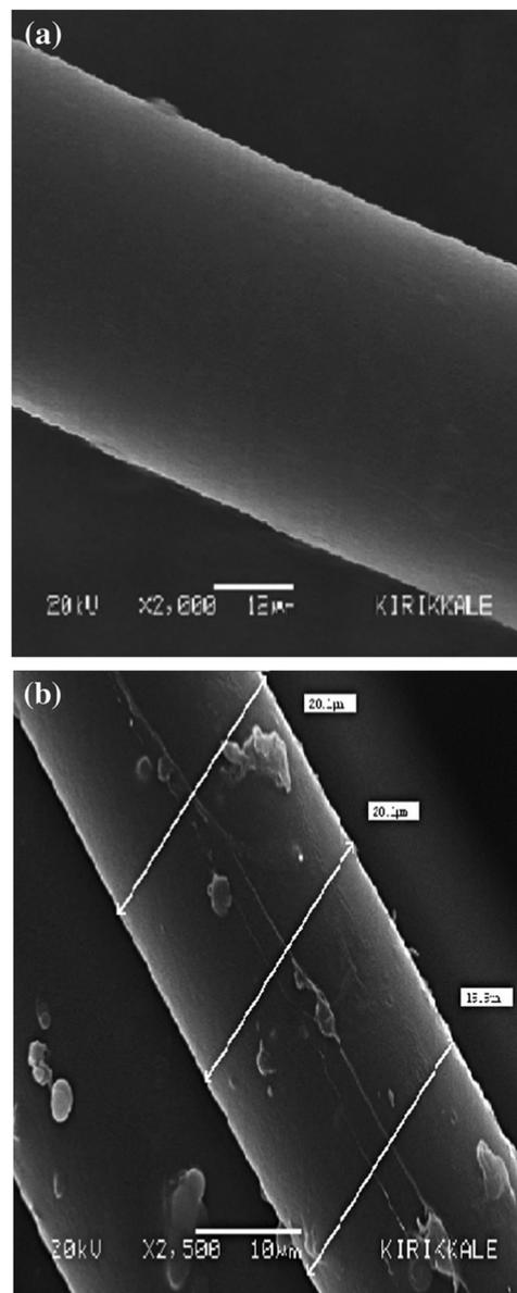
Fig. 15 SEM micrographs of (a) original PET fibers and (b) GMA-grafted PET fibers (having 150% graft yield).<sup>123</sup> Reproduced from ref. 123, with permission from Springer Nature, 2021.
