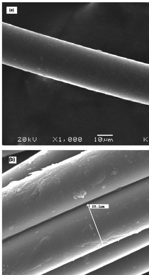
Fig. 19 (a) SEM micrograph of ungrafted PET fibers, and (b) SEM micrograph of MAA-GMA-grafted PET fibers (115%, 50/50 mol).<sup>139</sup> Reproduced from ref. 139, with permission from John Wiley and Sons, 2011.
