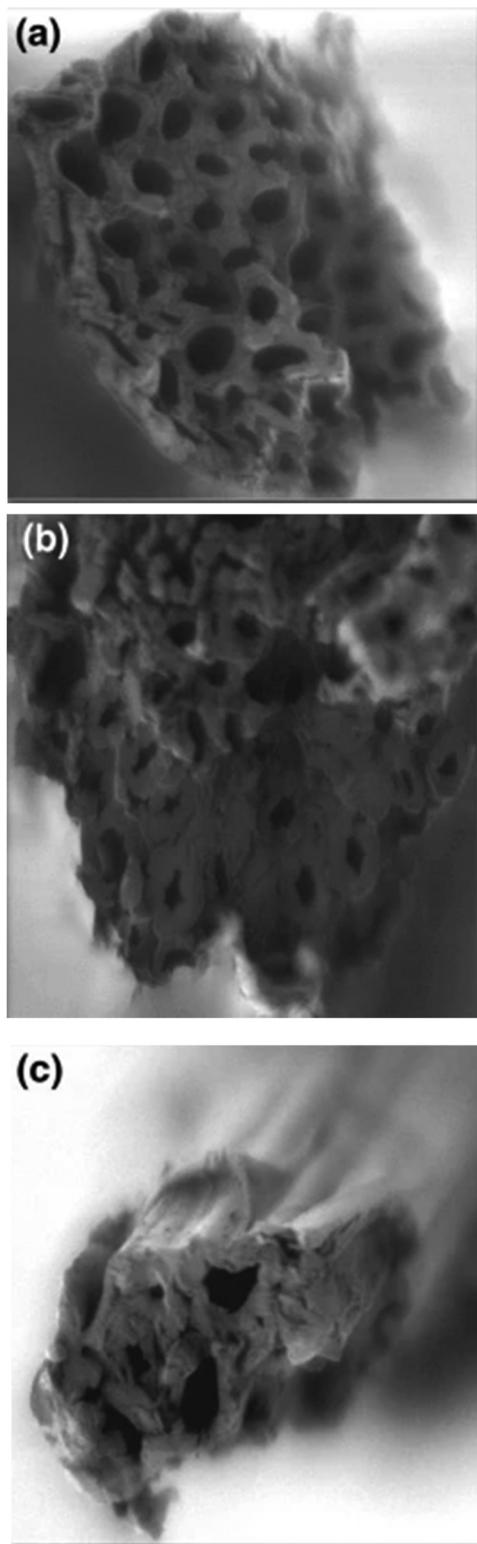
Fig. 16 FE-SEM cross-sectional images of hollow-centered banana trunk fiber for (a) GMA grafted fibers, (b) AFF, and (c) dye-loaded fibers with a magnification of  $\times 500$ .<sup>133</sup> Reproduced from ref. 133, with permission from Springer Nature, 2019.
