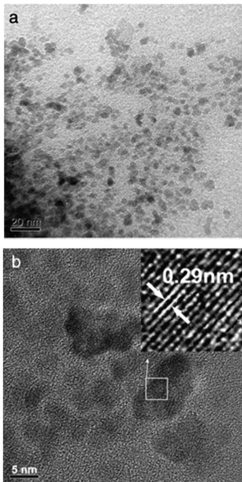
Fig. 7 TEM (a) and HR-TEM (b) images of  $MFe_3O_4$ -CS.<sup>64</sup> Reproduced from ref. 64, with permission from Elsevier, 2014.
