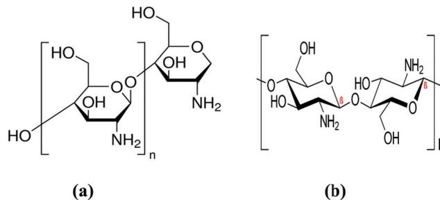
Fig. 2 (a) Chitosan; and (b)  $\beta$ -(1-4) chitosan structures.
