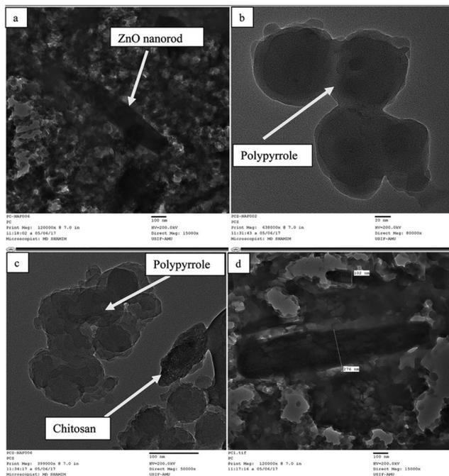
Fig. 4 TEM micrographs of the as-prepared nanoparticles and nanocomposites: (a) Pp-Z, (b) Pp, (c) Pp-CS, and (d) Pp-CS-Z.<sup>52</sup>
