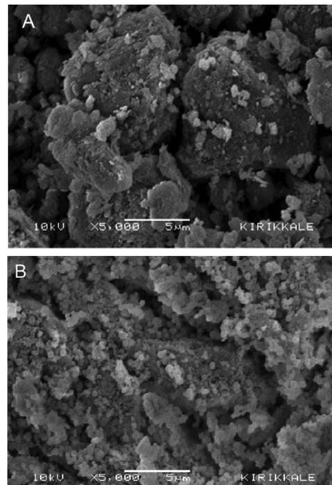
Fig. 17 SEM micrographs of different parts of samples at  $5000\times$  magnification. (A) natural zeolite, and (B) PGMA-Z-HMDA composite.<sup>134</sup> Reproduced from ref. 134, with permission from John Wiley and Sons, 2016.
