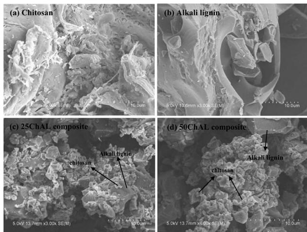
Fig. 10 SEM images of (a) CS, (b) AL, (c) 25-CS-AL composite, and (d) 50-CS-AL composite.<sup>79</sup> Reproduced from ref. 79, with permission from Elsevier, 2014.
