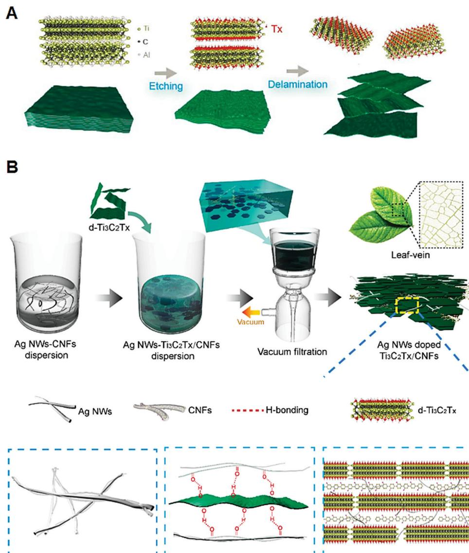
Fig. 5 (A) The preparative process for delaminated MXene nanosheets. (B) The production of the biomimetic silver (Ag) nanowires (NWs)-doped MXene ( $\text{Ti}_3\text{C}_2\text{T}_x$ )/cellulose nanofibrils (CNFs) films through a vacuum-assisted filtration technique. Reproduced with permission from ref. 72 Copyright 2021 Elsevier.
