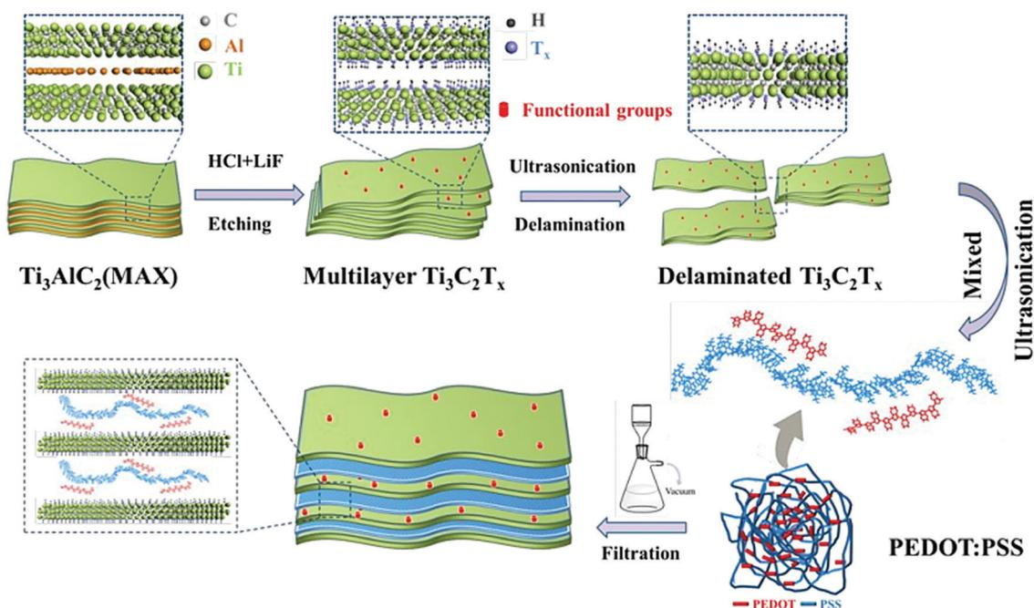
Fig. 4 The fabrication process for the bioinspired flexible composite films from  $\text{Ti}_3\text{C}_2\text{T}_x$  and poly(3,4-ethylenedioxythiophene)-poly(styrenesulfonate) (PEDOT:PSS) materials. Reproduced with permission from ref. 70 Copyright 2018 American Chemical Society.
