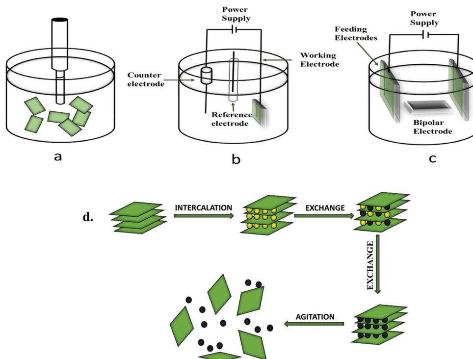
Fig. 3 Schematic representation of liquid-based exfoliation, (a) ultra-sonication, (b) electrochemical anodic or cathodic method, (c) bipolar electrochemical exfoliation method, and (d) schematic representation showing the exfoliation of BP nanosheets.
