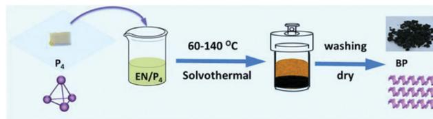
Fig. 5 Schematic representation of the synthesis of FLBP *via* the solvothermal process (reproduced from M. Pica and R. D'Amato, Chemistry of Phosphorene: Synthesis, Functionalization and Biomedical Applications in an Update Review. *Inorganics*, 2020, 8(4), 29.; published by MDPI, Basel, Switzerland). This article is an open access article distributed under the terms and conditions of the Creative Commons Attribution license (<https://doi.org/10.3390/inorganics8040029>).
