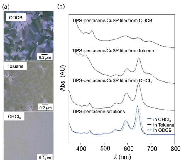
Fig. 3 (a) POM images of the TIPS-pentacene/CuSP blend films. (b) Absorption spectra of TIPS-pentacene/CuSP blend films and TIPS-pentacene solutions.
