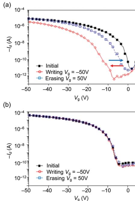
Fig. 5 Transfer characteristics of OFET memory devices fabricated using (a) TIPS-P/CuSP blend films and (b) TIPS-P/PS<sub>4</sub> blend films monitored at  $V_d = -50 \text{ V}$ .
