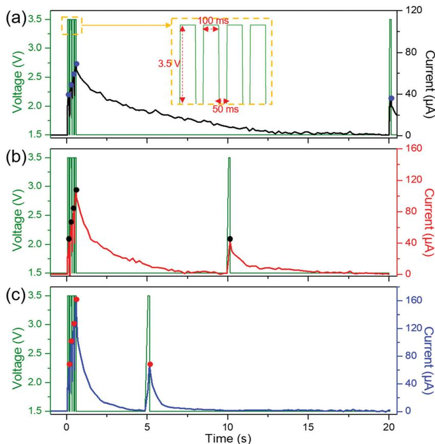
Fig. 6 Emulating the short-term synaptic plasticity. The current change was measured while applying 4 + 1 presynaptic spikes on (a) Device-P, (b) Device-1S, and (c) Device-2S.
