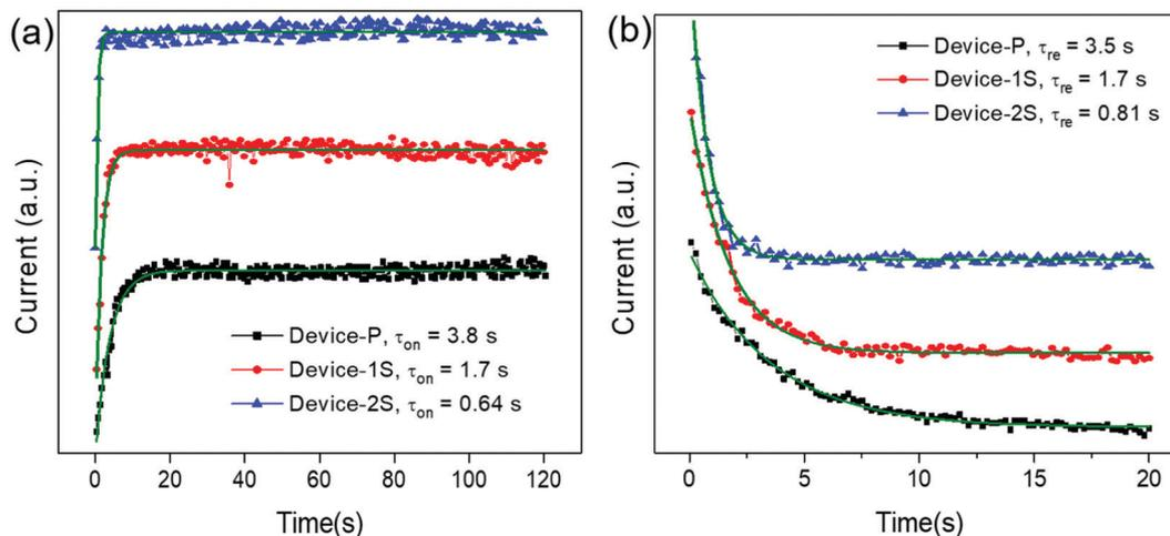
Fig. 4 Time-dependent current spectra for (a) turn-on time and (b) relaxation time of Device-P (black squares), Device-1S (red circles), and Device-2S (blue triangles) as indicated. The acquired turn-on time and relaxation time data were fitted to eqn (1) and (2), respectively, indicated with solid green lines.
