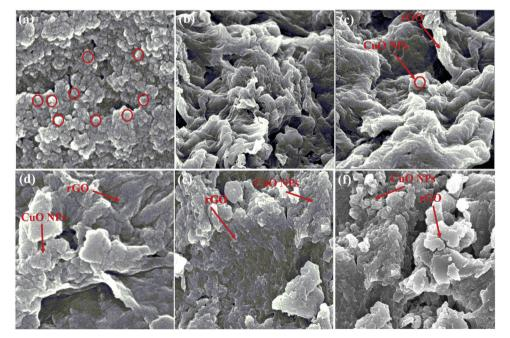
Fig. 3 FESEM photographs of (a-f) CG-I-CG-VI nanocomposites.
