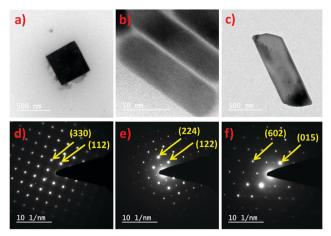
Fig. 4 (a) TEM image of square-shaped nanoplates of Cs<sub>2</sub>CuCl<sub>4</sub> at 500 nm scale bar. (b) TEM image of Cs<sub>2</sub>CuBr<sub>4</sub> nanorods at 50 nm scale bar. (c) TEM image of rectangular-shaped nanoplates of Cs2CuBr2Cl2 at 500 nm scale bar. (d) SAED pattern of Cs<sub>2</sub>CuCl<sub>4</sub> nanoplates. (e) SAED pattern of Cs<sub>2</sub>CuBr<sub>4</sub> nanorods. (f) SAED pattern of Cs<sub>2</sub>CuBr<sub>2</sub>Cl<sub>2</sub> nanoplates.
