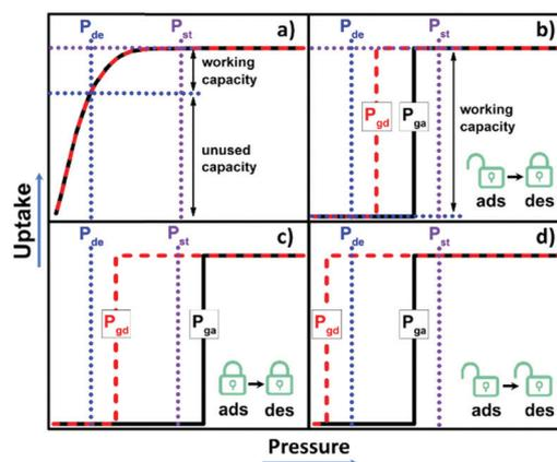
**Scheme 1** Comparison of different types of gas sorption isotherms. (a) type I; (b) type F-IV ( $P_{de} < P_{gd} < P_{ga} < P_{st}$ ); (c) type F-IV ( $P_{de} < P_{gd} < P_{st} < P_{ga}$ ) and (d) type F-IV ( $P_{gd} < P_{de} < P_{ga} < P_{st}$ ). Black solid line: adsorption; red dash line: desorption;  $P_{ga}$ : gate adsorption pressure;  $P_{gd}$ : gate desorption pressure;  $P_{de}$ : delivery pressure;  $P_{st}$ : storage pressure; ads: adsorption; des: desorption.
