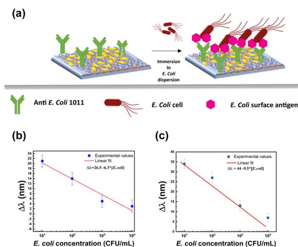
Fig. 7 Schematic of the mechanism of capturing *E. coli* cells promoted by the Ab incorporated on the plasmonic substrate. (a) Optical shift ( $\Delta\lambda$ ) as a function of *E. coli* concentration in the incubation dispersion, reported on a logarithmic scale for *E. coli* recognition experiments in the presence of SYTO 9™ (b) and in the absence of SYTO 9™ (c).
