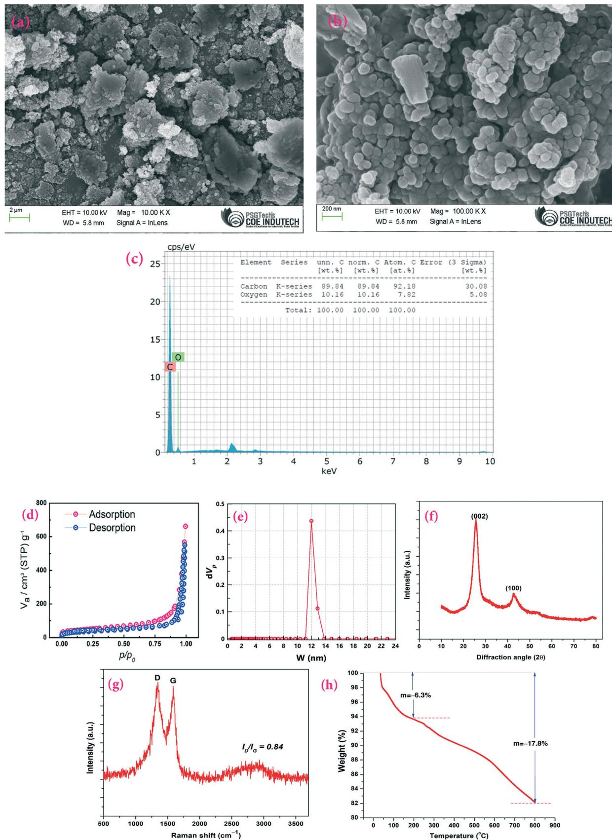
Fig. 3 Characterization of the produced CSCNP using SEM micrographs at magnifications of (a) 2  $\mu\text{m}$  and (b) 200 nm; (c) EDX analysis showing the percentage of the elements present; (d)  $\text{N}_2$  adsorption/desorption isotherm; (e) NLDFT/GCMC pore size distribution analysis; (f) XRD diffractogram; (g) Raman spectrum; and (h) thermogravimetric analysis.
