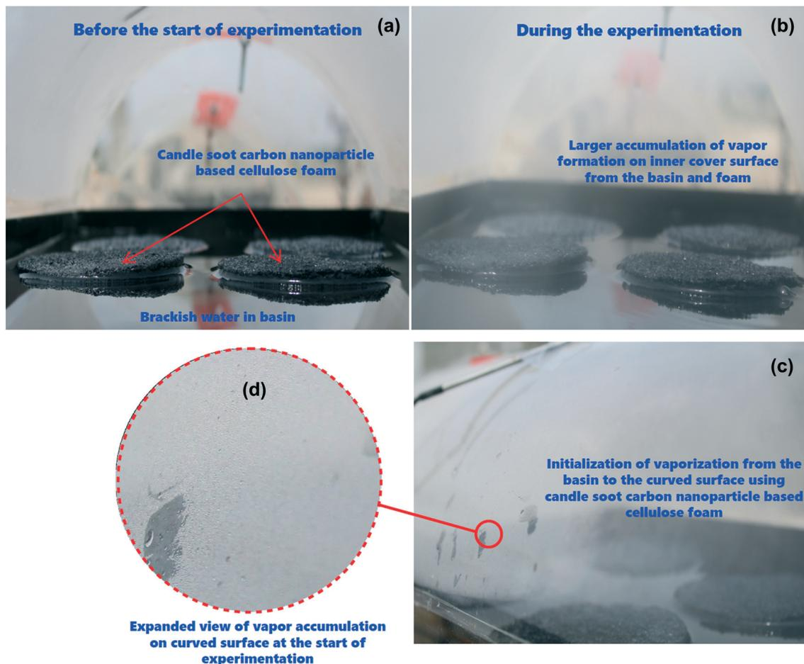
**Fig. 8** Initial stages of evaporation and condensation of water-droplets on the TSS cover. (a) Modified CSCNP foam is placed in the evaporation/condensation chamber of the TSS before the start of the experiment; (b) occurrence of evaporation in the initial stage of experimentation; (c) condensed water droplets accumulated on the cover at the beginning of the experiment; and (d) an enlarged view of the small sized droplet formation on the TSS cover.
