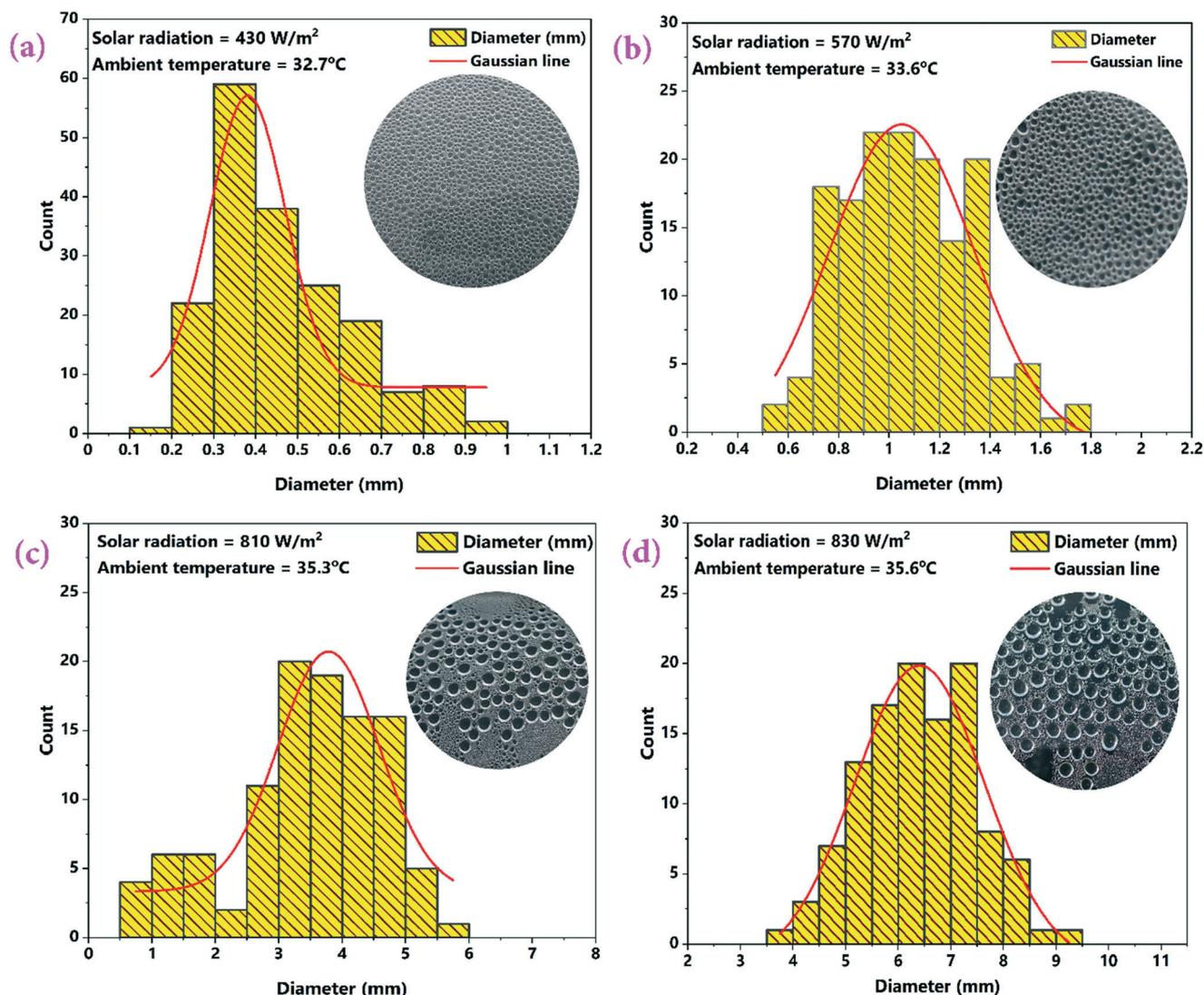
Fig. 9 Effect of varying solar radiation intensity on the condensed water-droplet formation inside the cover of the CSCNP-CF-TSS. (a) 430 W m<sup>-2</sup>, (b) 570 W m<sup>-2</sup>, (c) 810 W m<sup>-2</sup> and (d) 830 W m<sup>-2</sup>. The insets show the actual droplet sizes (photographs).
