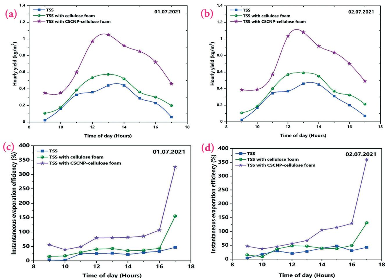
Fig. 11 (a and b) Hourly water yield, and (c and d) Instantaneous evaporation efficiency of the unmodified, CF-modified and CSCNP-CF modified TSS on 1st and 2nd July, 2021.
