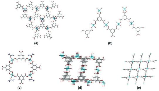
Fig. 8 Motifs observed for simple btc coordination polymers. (a) Hexagonal network, illustrated by ADOLUB, 48 (b) 2D tape, illustrated by TOPMIU,<sup>49</sup> (c) discrete quadrilateral motif, illustrated by OXAWOB,<sup>50</sup> (d) quadrilateral spiral network, illustrated by JEQNUP,<sup>51</sup> and (e) square-grid network, illustrated by MITRUD.52
