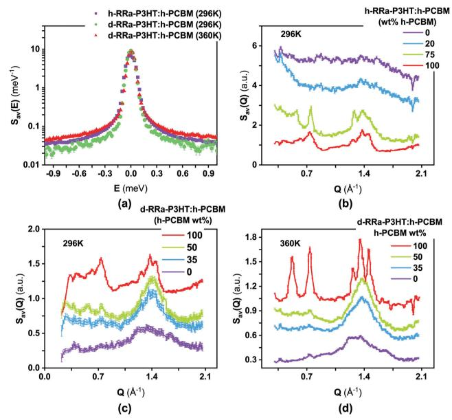
Fig. 4 (a) Q-Averaged QENS spectra at the miscibility limit. (b) Concentration-dependent neutron diffraction patterns of h-RRa-P3HT:h-PCBM at 296 K. (c) and (d) concentration-dependent neutron diffraction patterns of d-RRa-P3HT:h-PCBM at 296 K and 360 K, respectively
