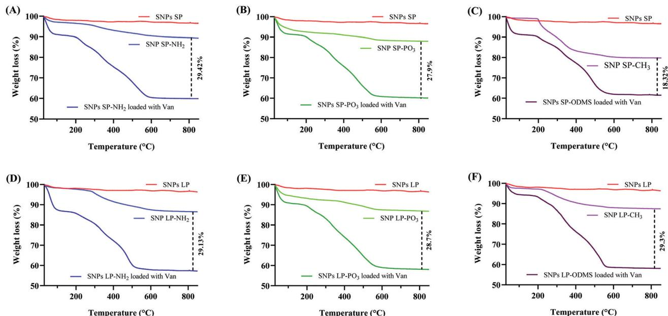
Fig. 6 TGA of (A) SNPs SP-NH<sub>2</sub> loaded with Van, (B) SNPs SP-PO<sub>3</sub> loaded with Van, (C) SNPs SP-CH<sub>3</sub> loaded with Van, (D) SNPs LP-NH<sub>2</sub> loaded with Van, (E) SNPs LP-PO<sub>3</sub> loaded with Van, and (F) SNPs LP-CH<sub>3</sub> loaded with Van.
