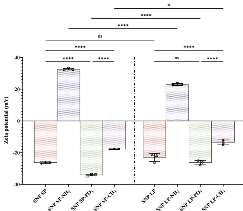
Fig. 2 Surface charge of SNPs with/without functional groups. Values are presented as mean  $\pm$  standard deviation ( $n = 3$ ). One-way ANOVA with Tukey's multiple comparisons test was performed. ns: no significance; significance level was \* $p < 0.033$ , \*\*\*\* $p < 0.0001$ .
