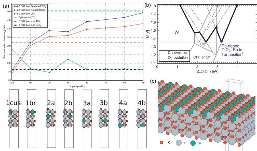
Fig. 5 (a) Covered oxygen adsorption energy  $\Delta E(\text{O}_2)$  for Ru-doped  $\text{TiO}_2$ , Ti-doped  $\text{RuO}_2$ , DSA and pure  $\text{RuO}_2$  and  $\text{TiO}_2$  at different dopant positions from DFT modelling. (b) Volcano plot from Hansen's work in collaboration with Ru-doped  $\text{TiO}_2$  at the '1b' site (bold line) in this work. (c) A unit model of the optimized identical Ru-doped  $\text{TiO}_2$  surface. Reproduced with permission.<sup>56</sup> Copyright 2014, Elsevier.
