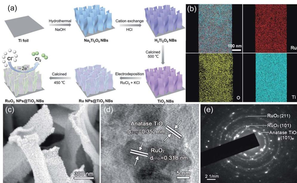
Fig. 10 (a) Schematic diagram of the  $\text{RuO}_2$  NPs@ $\text{TiO}_2$  NB synthesis process. (b) Energy-dispersive X-ray spectroscopy (EDX) images of  $\text{RuO}_2$  NPs@ $\text{TiO}_2$  NBs. (c) SEM images of  $\text{RuO}_2$  NPs@ $\text{TiO}_2$  NBs. (d) TEM images and (e) SAED analysis of  $\text{RuO}_2$  NPs@ $\text{TiO}_2$  NBs. Reproduced with permission.<sup>48</sup> Copyright 2020, Elsevier.
