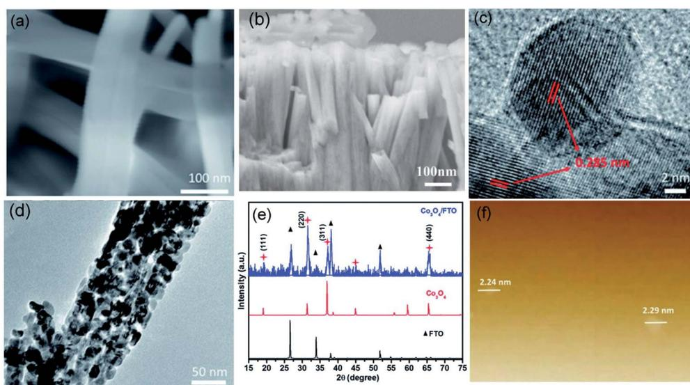
Fig. 13 (a and b) SEM images of  $Co_3O_4$  nanobelt morphologies on the fluorine doped tin oxide (FTO) substrate. (c and d) TEM images of  $Co_3O_4$  NBAs on the FTO substrate. (e) XRD comparison of the  $Co_3O_4/FTO$ ,  $Co_3O_4$  and FTO. (f) AFM images of the  $Co_3O_4$ . Reproduced with permission.<sup>17</sup> Copyright 2018, Royal Society of Chemistry.
