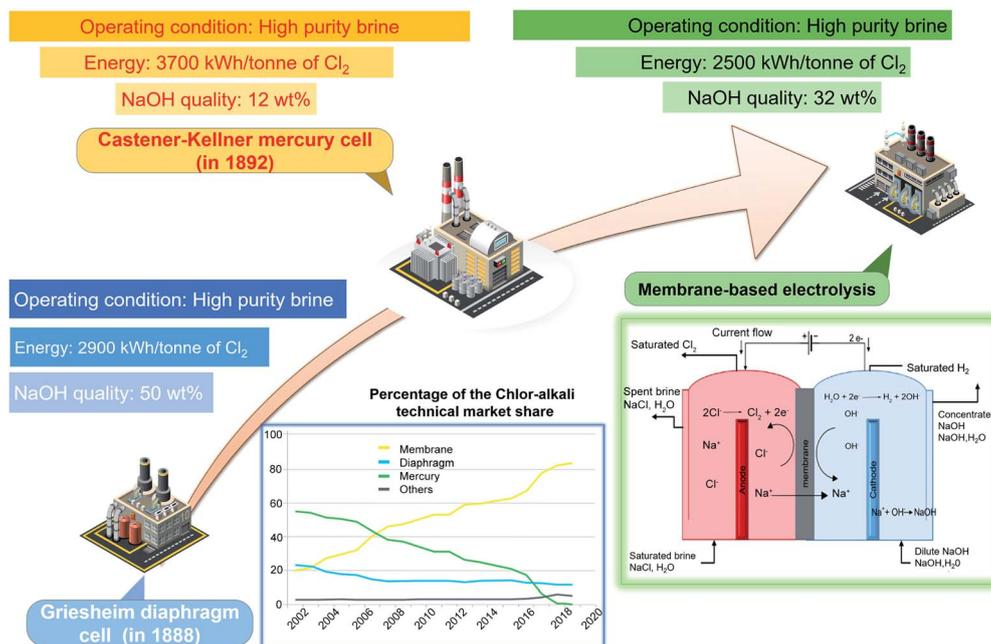
Fig. 1 Comparison of the diaphragm, mercury, and membrane cell in the chlor-alkali process. Reproduced with permission.<sup>20</sup> Copyright 2019, Elsevier.
