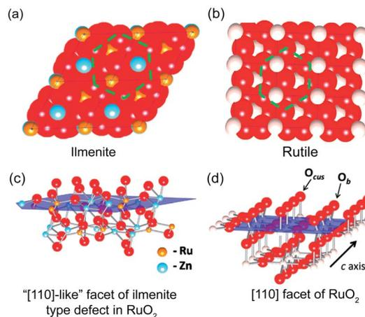
Fig. 6 (a) Atomic close packing model of the ilmenite structure and (b) rutile structure. (c) Spatial ilmenite structure of the active RuO<sub>2</sub> (110) surface. (d) Spatial rutile structure of the active RuO<sub>2</sub> (110) surface. Reproduced with permission.<sup>44</sup> Copyright 2011, American Chemical Society.
