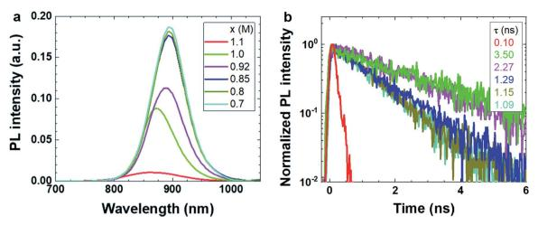
Fig. 4 PL measurements of PEA<sub>0.08</sub>FA<sub>x</sub>SnI<sub>3</sub> films. (a) Steady state and (b) time-resolved PL. The color scheme is the same in the two figures, lifetimes are reported in the legend of (b).
