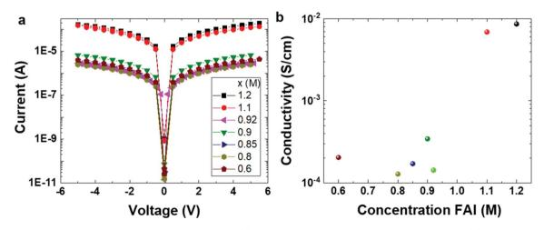
Fig. 5 Conductivity measurements of  $PEA_{0.08}FA_{(x)}SnI_3$  films. (a) I-V characteristics under dark conditions, and (b) electrical conductivity calculated from the I-V curves in (a)
