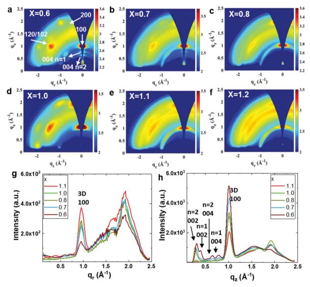
Fig. 2 GIWAXS patterns of (a) the PEA $_{0.08}$ FA $_{0.6}$ SnI $_3$ , (b) PEA $_{0.08}$ FA $_{0.7}$ SnI $_3$ , (c) PEA $_{0.08}$ FA $_{0.8}$ SnI $_3$ , (d) PEA $_{0.08}$ FA $_{1.0}$ SnI $_3$ , (e) PEA $_{0.08}$ FA $_{1.1}$ SnI $_3$  and (f)  $PEA_{0.08}FA_{1.2}Snl_3$  films. The images were recorded using an incident angle of 2°. Line-cut data of the  $PEA_{0.08}FA_xSnl_3$  (x = 0.6-1.1) films along (g)  $q_r$ and (h)  $q_z$  directions.
