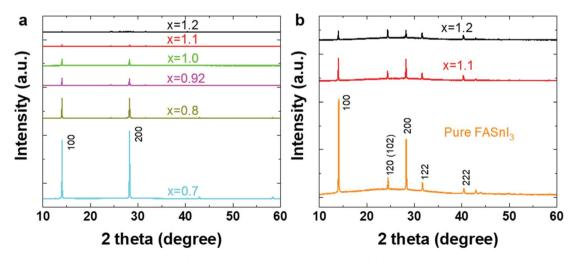
Fig. 1 XRD patterns of PEA $_{0.08}$ FA $_x$ SnI $_3$  films with (a) x ranging from 0.70 M to 1.20 M and (b) the 1.10 M and 1.20 M patterns compared to the one of pure FASnI $_3$ .
