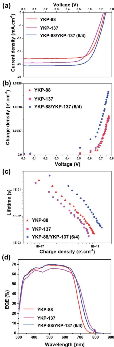
Fig. 5 (a) Current–voltage ( $J$ ,  $V$ ) curves for YKP-88, YKP-137 and YKP-88/YKP-137 (6/4) devices, (b) charge extraction data showing electron density as a function of induced voltage for the corresponding DSSCs (c) transient photovoltage data showing electron lifetimes versus electron density. (d) Comparison of the IPCE spectra of YKP-88-, YKP-137-based solar cells and the co-sensitized device (ratio 6/4).
