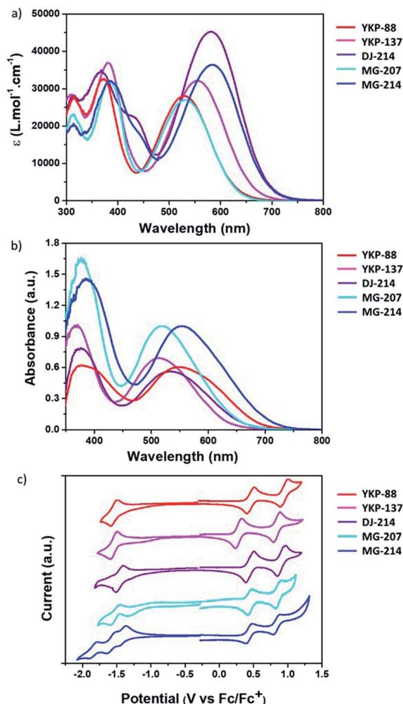
Fig. 3 (a) Absorption spectra registered (a) in Dichloromethane solution, (10<sup>-5</sup> M, 25 °C), (b) on 2 μm-thick mesoporous TiO<sub>2</sub> electrodes, for compounds YKP-88 (red line), YKP-137 (magenta line), DJ-214 (violet line) MG-207 (cyan line) and MG-214 (blue line) (c) cyclic voltammetry traces in solution for each compound (deoxygenated dichloromethane, 10<sup>-3</sup> M, 25 °C, voltage scan 200 mV s<sup>-1</sup>).
