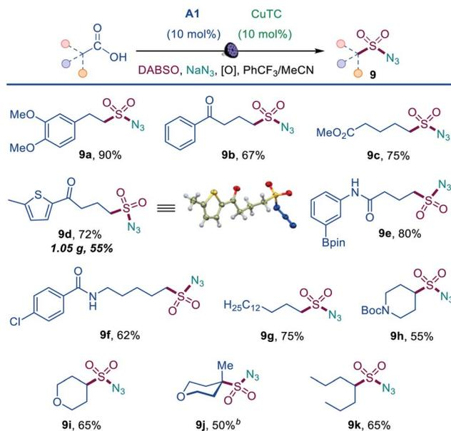
**Scheme 3** Scope of the direct decarboxylative azidosulfonation. Reaction conditions: carboxylic acid (0.3 mmol), copper 2-thiophenecarboxylate (CuTC) (10 mol%), **A1** (10 mol%), DABSO (0.45 mmol), <sup>t</sup>BuO<sub>2</sub>Bz (0.75 mmol), NaN<sub>3</sub> (0.9 mmol), PhCF<sub>3</sub>/MeCN (3 : 1, 3 mL), LED light (400 nm), 12 h.
